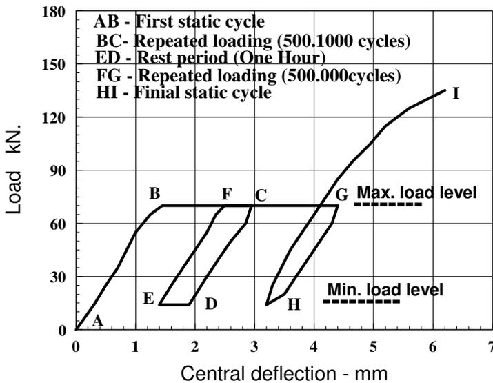
**Fig.2:** Sketch of sequence of loading versus deflection (Repeated tests)
