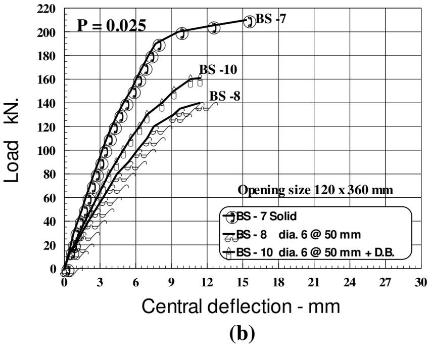
Fig. 6: Effect of using diagonal bars.
