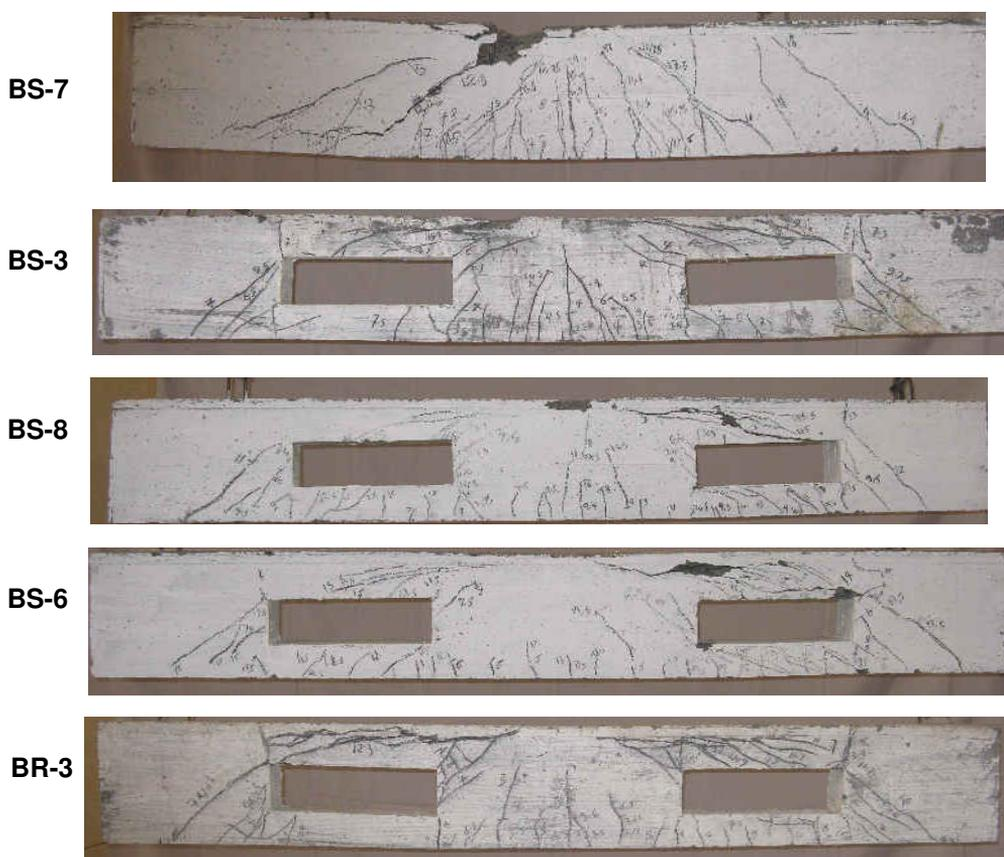
**Fig.3:** Failure patterns of some test beams
