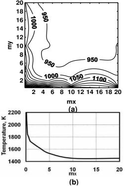
Fig. 3 Variation of maximum temperatures, in Kelvin, for the adopted  $ZrO_2/6061$ -T6/Ti-6Al-4V 2D-FGM plates where the maximum value is 2200 K. (a) For different values of  $m_x$  and  $m_y$ . (b) For different values of  $m_x$  and  $m_y = 0$ .
