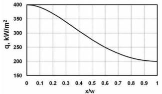
Fig. 2. Non-uniform heat flux that applied on the upper surface of the ZrO<sub>2</sub>/6061-T6/Ti-6A1-4V 2D-FGM plate.
