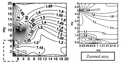
Fig. 6 Variations of the maximum normalized equivalent stresses that resulted in  $ZrO_2/6061$ -T6/Ti-6Al-4V 2D-FGM plates versus the values of the nonhomogenous parameters  $m_x$  and  $m_y$  during heating stage where the maximum and minimum values are 2.0 and 0.8 respectively.
