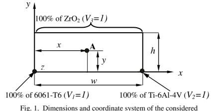
ZrO<sub>2</sub>/6061-T6/Ti-6Al-4V 2D-FGM plate.
