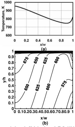
Fig. 5 Temperature variations, in Kelvin, through  $ZrO_2/6061$ -T6/Ti-6Al-4V 2D-FGM plate for  $m_x = 10$  and  $m_y = 10$  where the maximum value of temperature is 950 K. (a) Through upper surface of the plate. (b) Through the whole of the plate.
