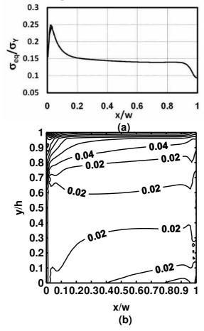
Fig. 9 Variation of the maximum normalized von Mises equivalent stresses  $\sigma_{eq}/\sigma_{Y}$ , for the optimum case ( $m_x = 0.1$  and  $m_y = 5$ ) during cooling stage that was achieved after staring of cooling process where the maximum value is about 0.24. (a) Through upper surface of the plate. (b) Through the whole of the plate.
