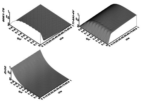
Fig. 10 Variations of the optimum composition of the three basic constituents of  $ZrO_2/6061$ -T6/Ti-6Al-4V 2D-FGM, for  $m_x = 0.1$  and  $m_y = 5$ .
