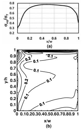
Fig. 8 Variation of the maximum normalized von Mises equivalent stresses  $\sigma_{eq}/\sigma_Y$ , for the optimum case (m<sub>x</sub> = 0.1 and m<sub>y</sub> = 5) during heating stage that was achieved at steady state where the maximum value is 0.8. (a) Through upper surface of the plate. (b) Through the whole of the plate.
