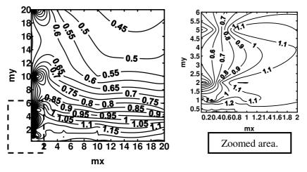
Fig. 7 Variations of the maximum normalized equivalent stresses that resulted in  $ZrO_2/6061$ -T6/Ti-6Al-4V 2D-FGM plates versus the values of the nonhomogenous parameters  $m_x$  and  $m_y$  during cooling stage where the maximum and minimum values are 1.3 and 0.24 respectively.
