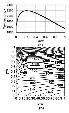
Fig. 4 Temperature variations, in Kelvin, through  $ZrO_2/6061$ -T6/Ti-6Al-4V 2D-FGM plate for  $m_x = 0.1$  and  $m_y = 0.1$  where the maximum value of temperature is 2200 K. (a) Through upper surface of the plate. (b) Through the whole of the plate.
