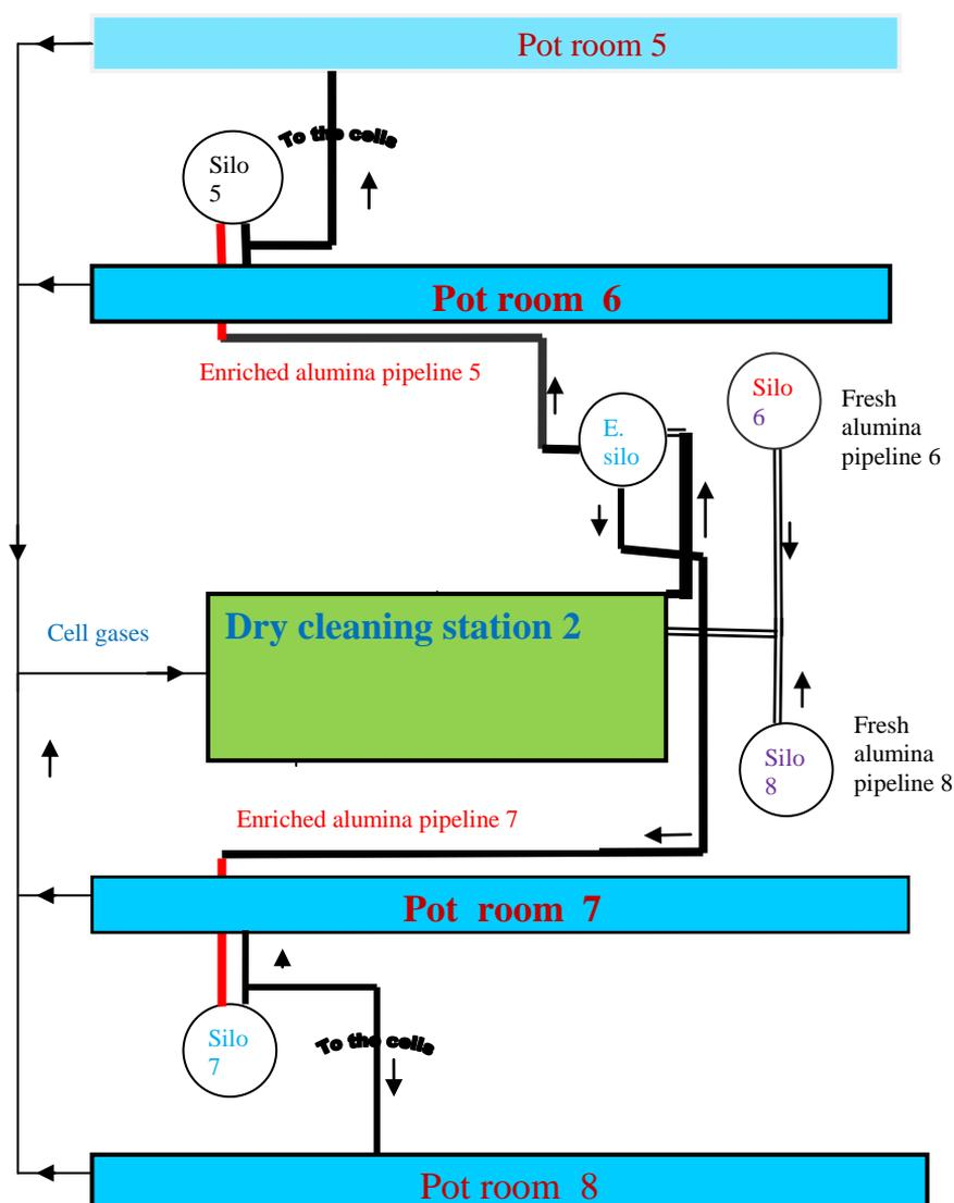
Fig.2: Schematic diagram for the Soderberg pipeline system
