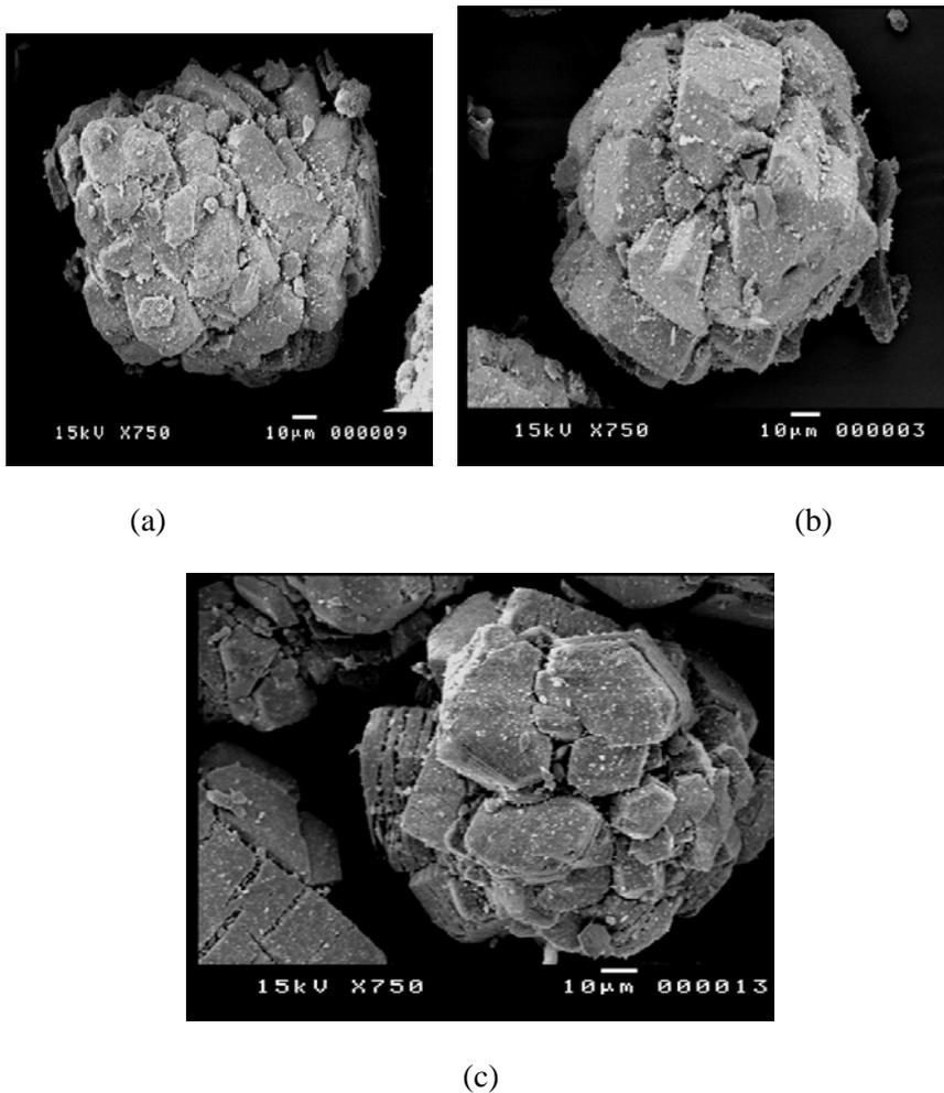
Fig.4: SEM photographs of the enriched alumina used in the Soderberg system (a), enriched alumina used in pre-baked system (b) and fresh alumina (c)
