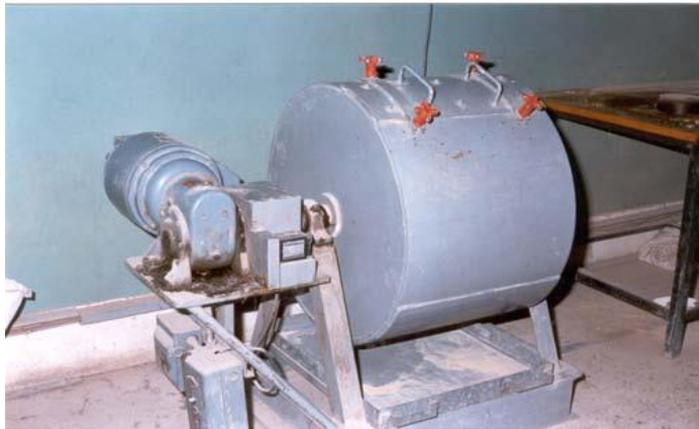
Figure 3: Los Angeles abrasion apparatus
