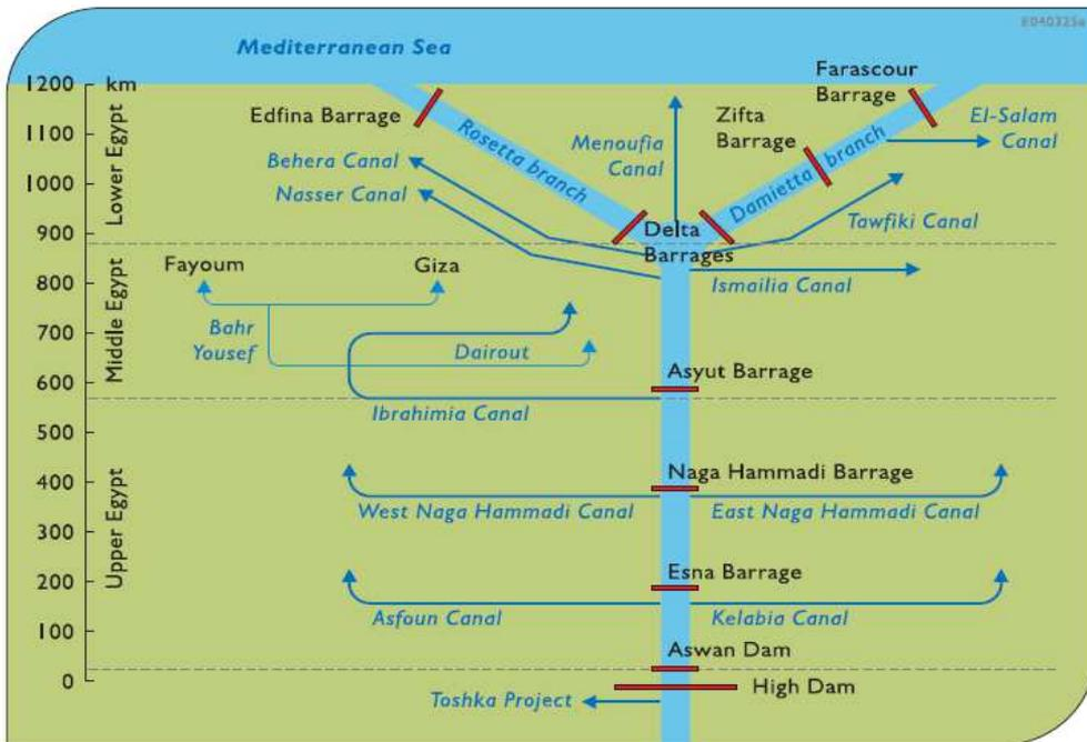
Fig. 2. Schematic diagram of major control structure on the Nile in Egypt [8]
