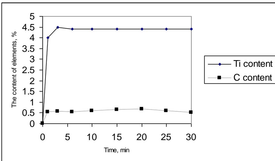
Fig. 8. The relationship between the reaction time and the content of Ti and C in Al-Ti-C master alloys at constant temp. = 1000 °C, R= 0.25 and  $R_1= 0.01$ .
