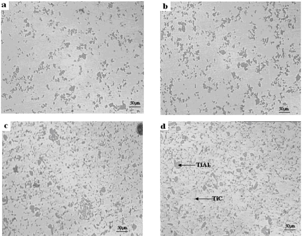
Fig. 5. Optical photomicrographs of the produced Al-Ti-C master alloys at 20 min and various temperatures.
