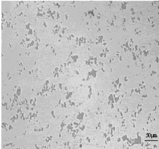
Fig. 1. Optical photomicrograph of the produced Al-4.3Ti-0.55C master alloy at 800°C
