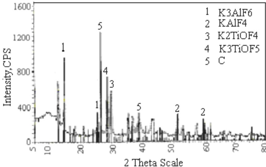
Fig. 4. XRD analysis of slag sample, at 1000°C and 20min
