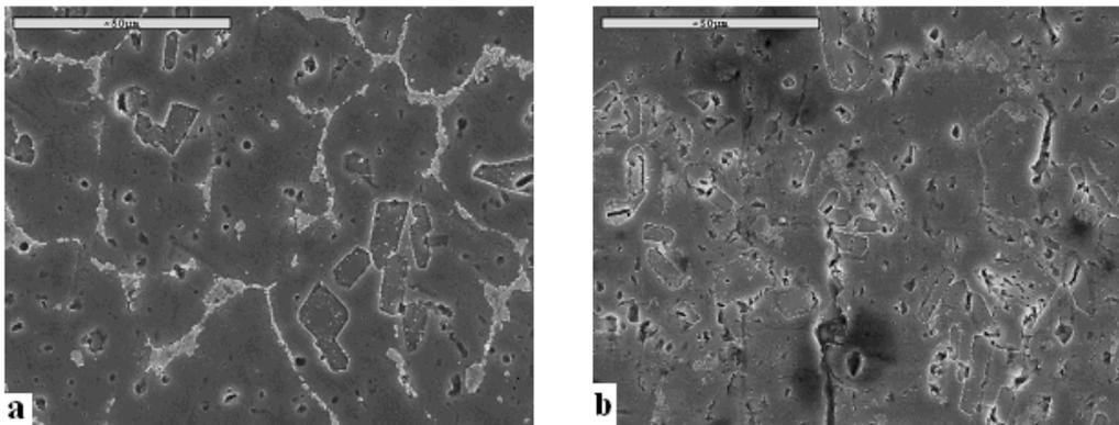
Fig. 6. SEM photomicrographs of the produced Al-Ti-C master alloys at 1000 °C and different reaction times.
