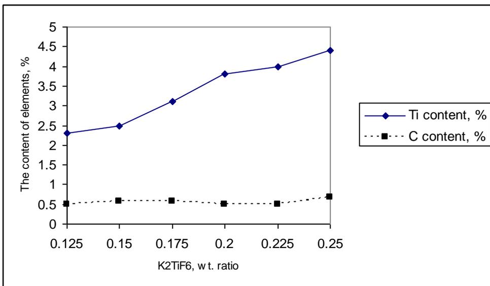
Fig. 7. The relationship between the  $K_2TiF_6/Al$  weight ratio and the content of Ti and C in Al-Ti-C master alloys at constant temp. = 1000 °C, time = 20 min and  $R_1= 0.01$ .
