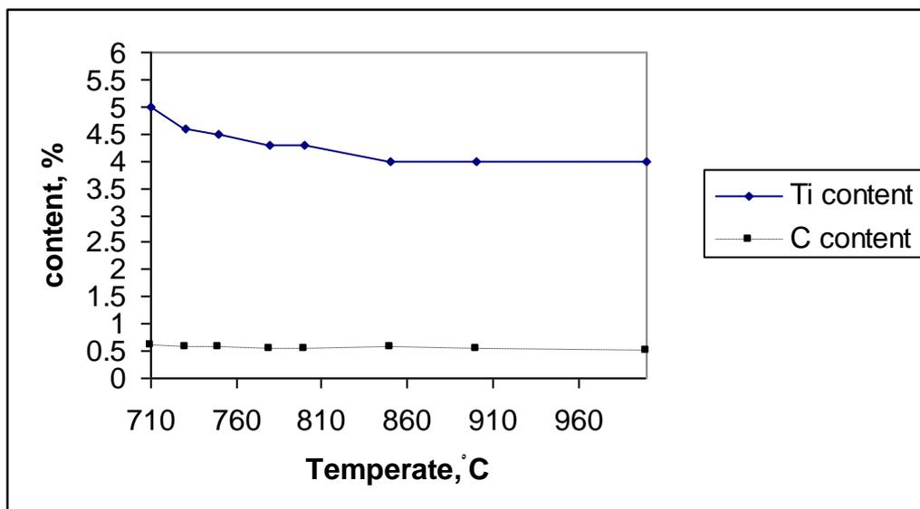
Fig. 9. The relationship between the reaction temperature and the content of Ti and C in the Al-Ti-C master alloys at constant time = 20min,  $R = 0.225$  and  $R_1 = 0.01$ .
