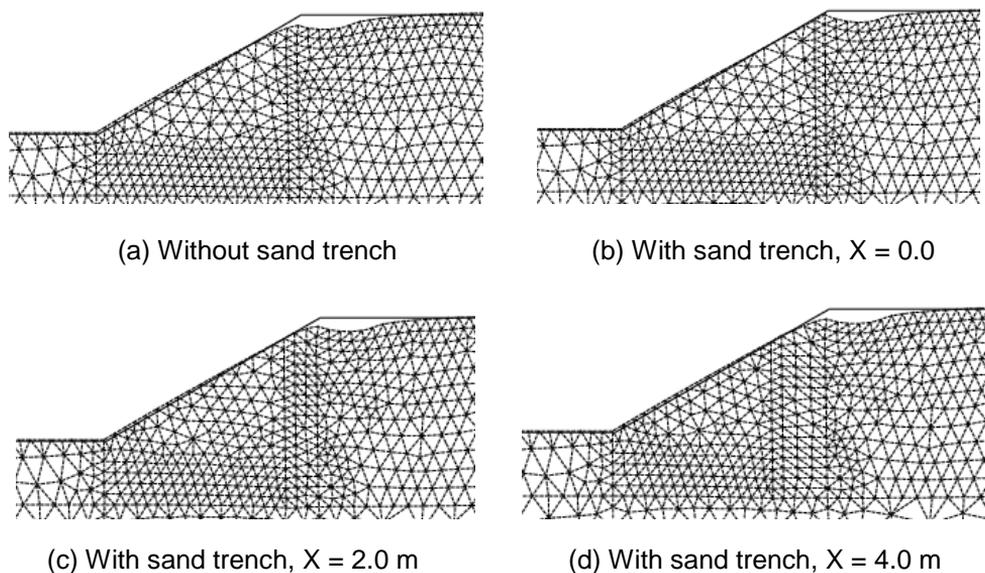
**Figure 4.** Deformation shapes for slope ( $\beta = 30^\circ$ ) due to strip footing, case of soft clay ( $C = 10 \text{ KN/m}^2$ )
