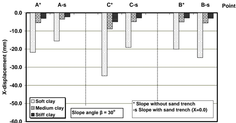
Figure 14. Comparison between additional horizontal displacements in slope ( $\beta = 30^\circ$ ) for different types of clay soil due to strip load.
