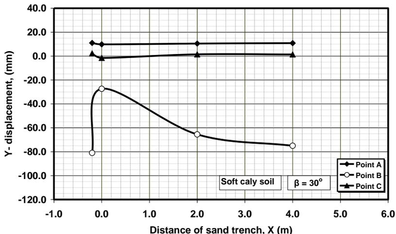
**Figure 10.** Vertical displacements for slope ( $\beta = 30^\circ$ ) due to strip footing, case of soft clay ( $C = 10 \text{ KN/m}^2$ )
