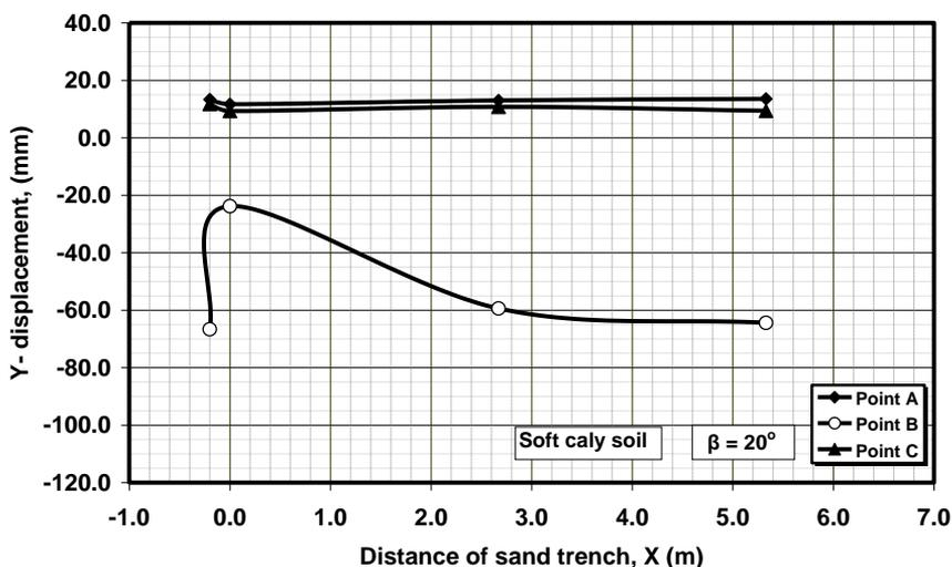
**Figure 11.** Vertical displacements for slope ( $\beta = 20^\circ$ ) due to strip footing, case of soft clay ( $C = 10 \text{ KN/m}^2$ )
