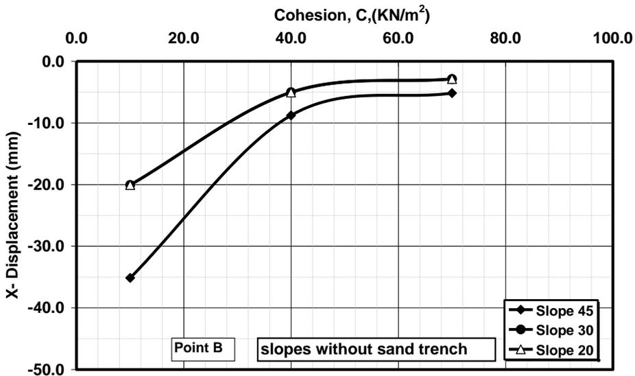
Figure 16. Additional horizontal displacements versus cohesion at point **B** for different slopes in the case of soil profiles without sand trench.
