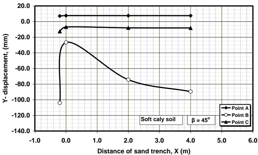
Figure 9. Vertical displacements for slope ( $\beta = 45^\circ$ ) due to strip footing, case of soft clay ( $C = 10 \text{ KN/m}^2$ )
