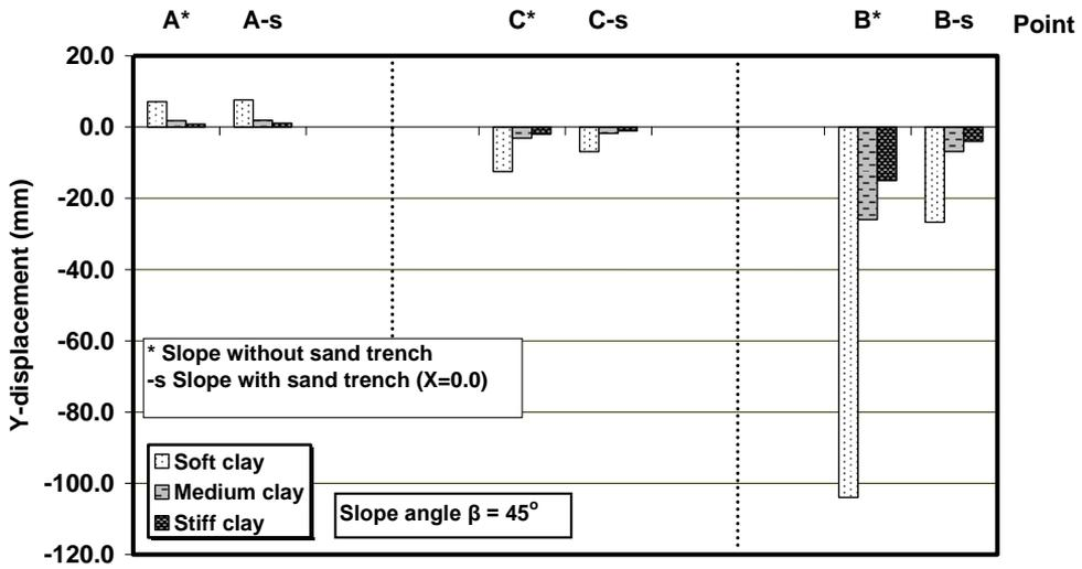
Figure 18. Comparison between additional vertical displacements in slope ( $\beta = 45^\circ$ ) for different types of clay soil due to strip load.
