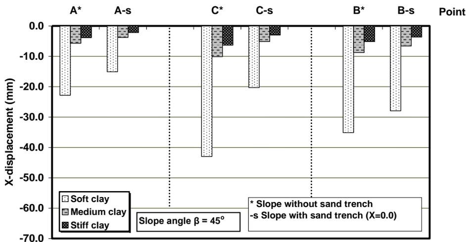
Figure 13. Comparison between additional horizontal displacements in slope ( $\beta = 45^\circ$ ) for different types of clay soil due to strip load.
