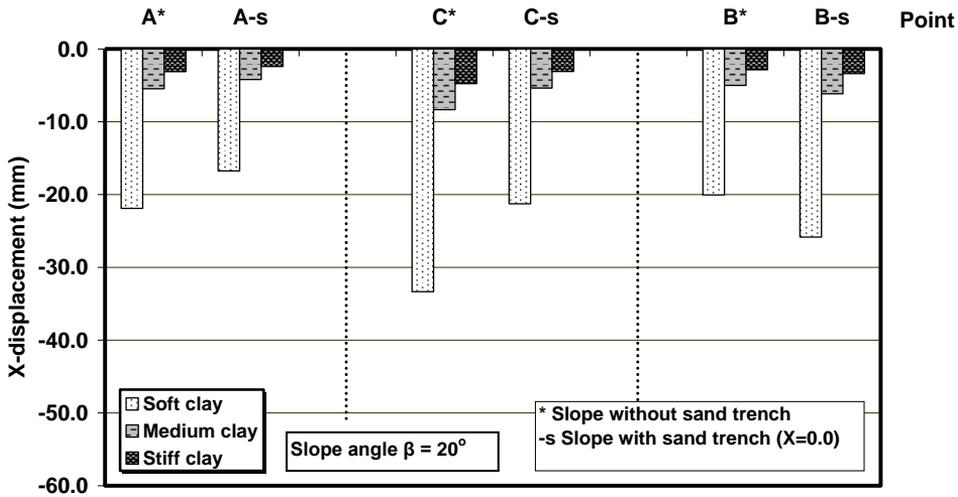
Figure 15. Comparison between additional horizontal displacements in slope ( $\beta = 20^\circ$ ) for different types of clay soil due to strip load.
