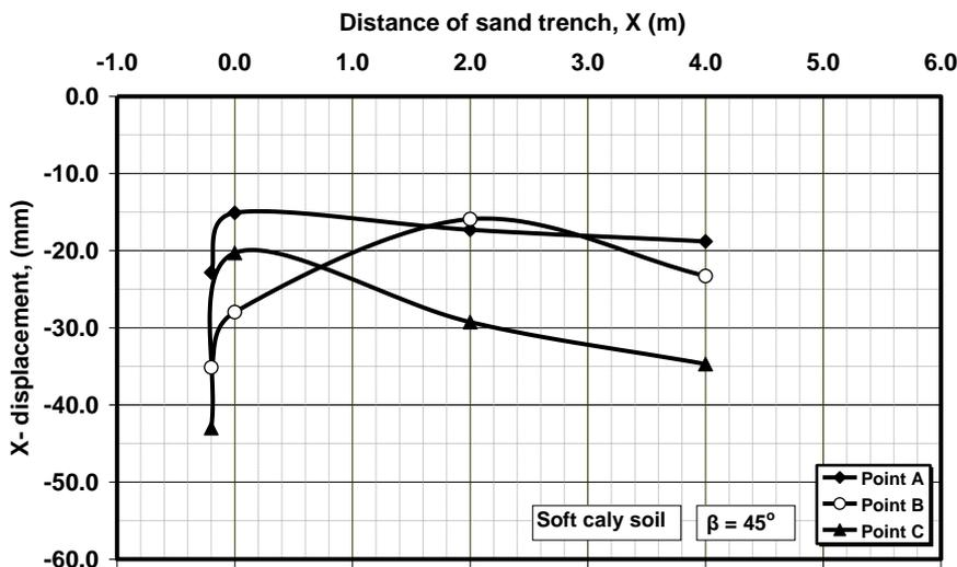
Figure 5. Horizontal displacements for slope ( $\beta = 45^\circ$ ) due to strip footing, case of soft clay ( $C = 10 \text{ KN/m}^2$ )
