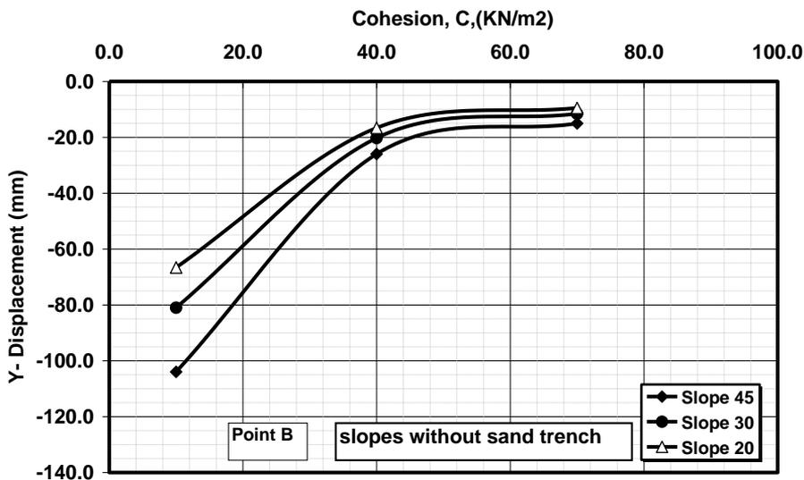
Figure 21. Additional vertical displacements versus cohesions at point B for different slopes in the case of soil profiles without sand trench.
