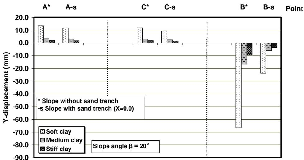
Figure 20. Comparison between additional vertical displacements in slope ( $\beta = 20^\circ$ ) for different types of clay soil due to strip load.
