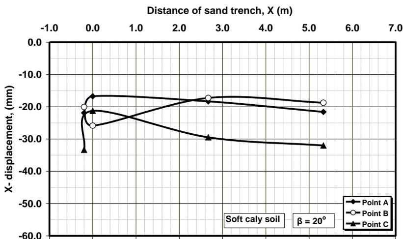
**Figure 7.** Horizontal displacements for slope ( $\beta = 20^\circ$ ) due to strip footing, case of soft clay ( $C = 10 \text{ KN/m}^2$ )
