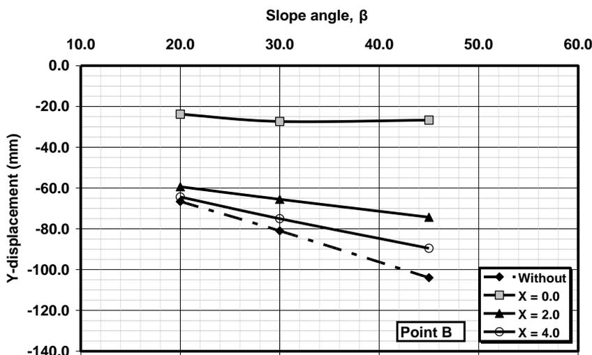
Figure 12. Vertical displacements versus slope angle  $\beta$  for point B due to strip footing, case of soft clay ( $C = 10 \text{ KN/m}^2$ )
