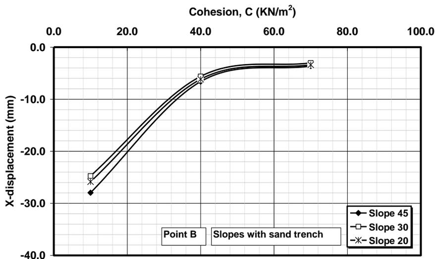
**Figure 17.** Additional horizontal displacements versus cohesions at point **B** for different slopes in the case of soil profiles with sand trench ( $X = 0.0$ ).
