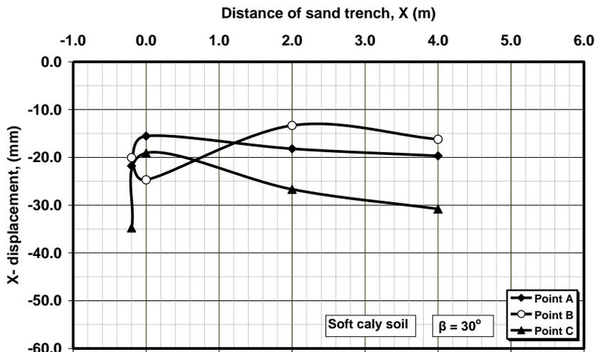
**Figure 6.** Horizontal displacements for slope ( $\beta = 30^\circ$ ) due to strip footing, case of soft clay ( $C = 10 \text{ KN/m}^2$ )
