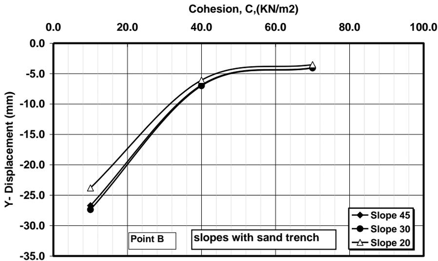
**Figure 22.** Additional vertical displacements versus cohesions at point **B** for different slopes in the case of soil profiles with sand trench ( $X = 0.0$ ).
