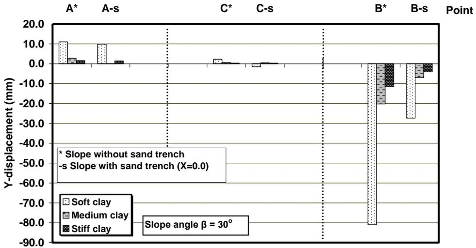
Figure 19. Comparison between additional vertical displacements in slope ( $\beta = 30^\circ$ ) for different types of clay soil due to strip load.
