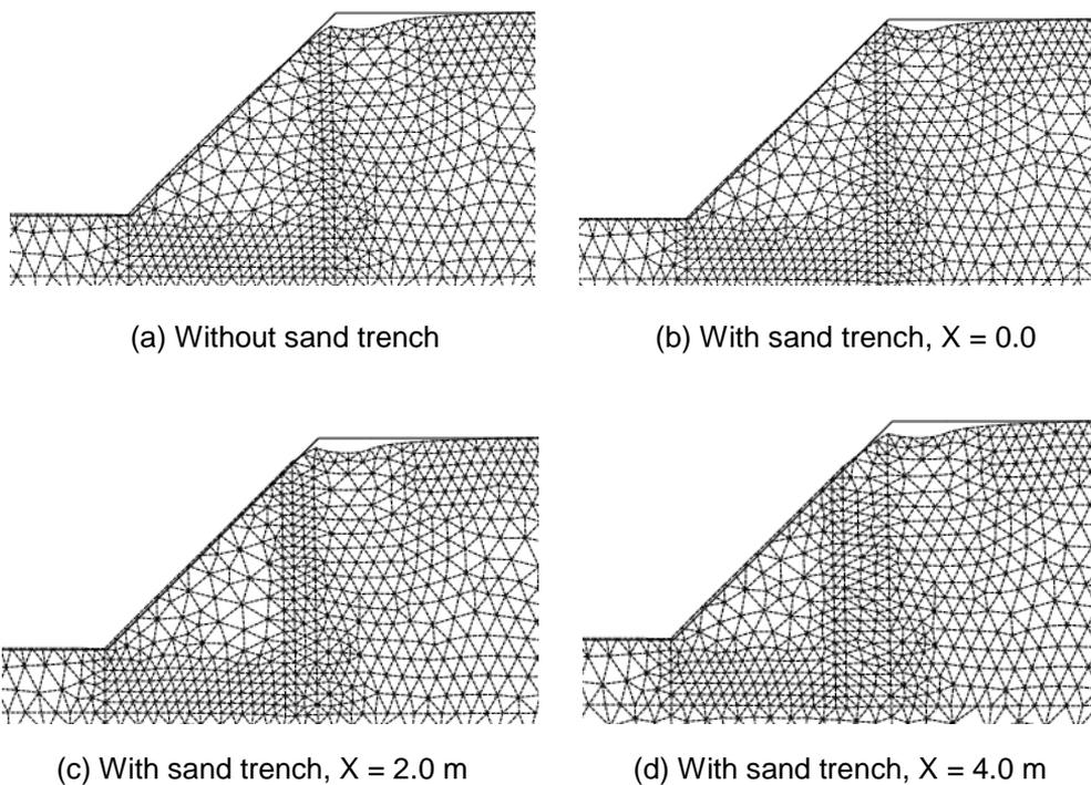
**Figure 3.** Deformation shapes for slope ( $\beta = 45^\circ$ ) due to strip footing, case of soft clay ( $C = 10 \text{ KN/m}^2$ )
