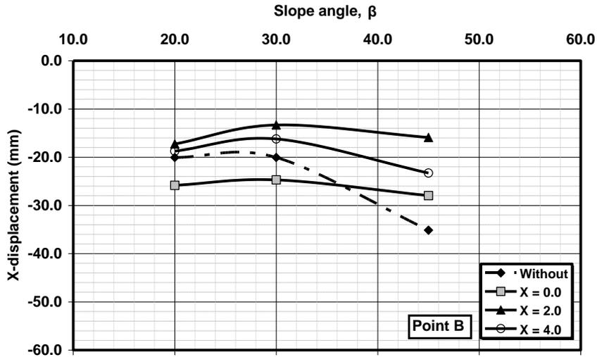
Figure 8. Horizontal displacements versus slope angle  $\beta$  for point B due to strip footing, case of soft clay ( $C = 10 \text{ KN/m}^2$ )
