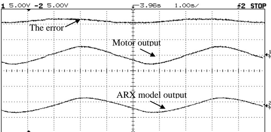
Fig. 10 The experimental motor and the ARX model outputs to a sawtooth wave input.
