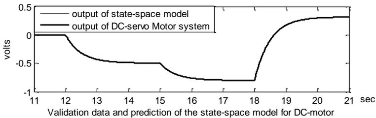
(c) DC-servo motor system and state space model outputs.
