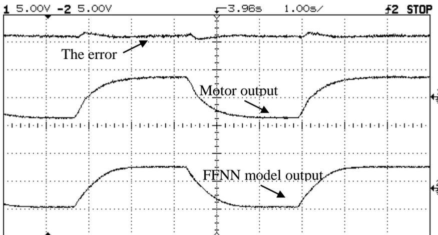
Fig. 13 The experimental motor and the neural network model outputs to a square wave input.
