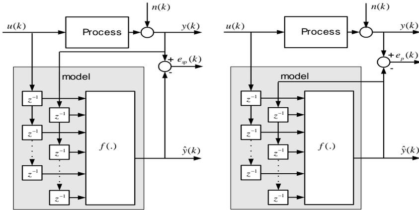
Fig. 5 (a) One-step prediction with a series parallel model
