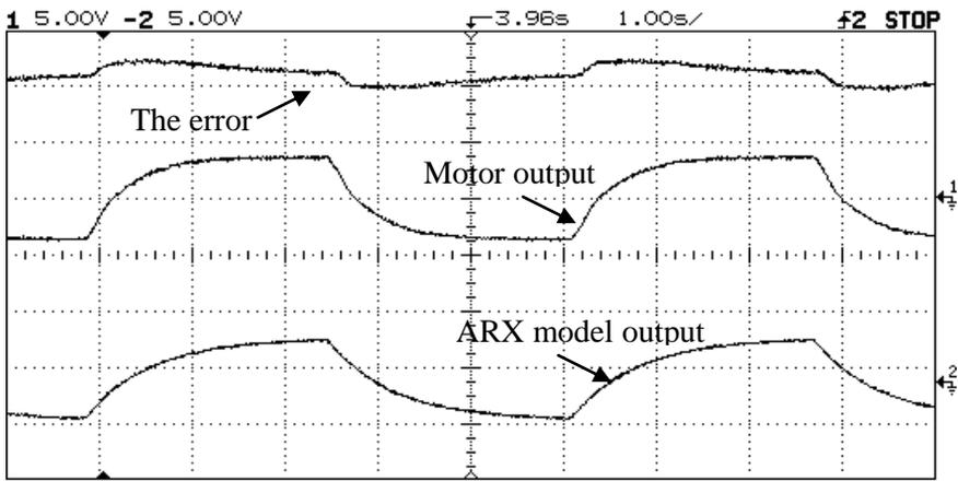
Fig. 9 The experimental motor and the ARX model outputs to a square wave input.
