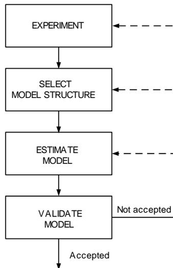
Fig. 2 The basic system identification procedure
