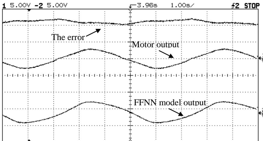
Fig. 14 The experimental motor and the neural network model outputs to a sawtooth wave input.
