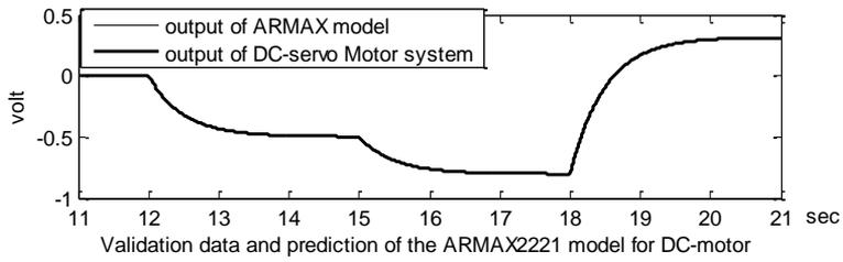
(b) DC-servo motor system and ARMAX model outputs.
