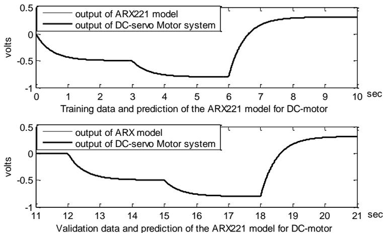
(a) DC-servo motor system and ARX model outputs.
