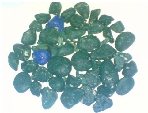
**Figure (1):** Coated aggregates with polypropylene
