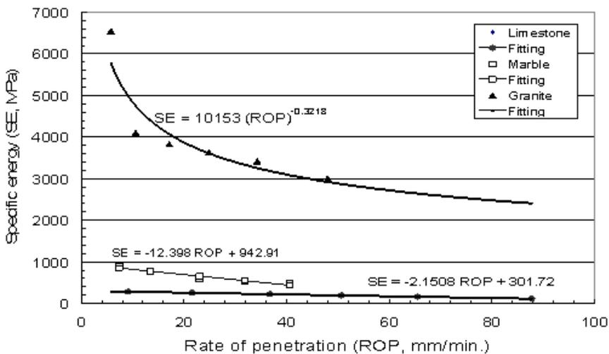
Figure (2) Relationship between average rate of penetration and specific energy for all rocks at different loads and drilling speed of 300 rpm
