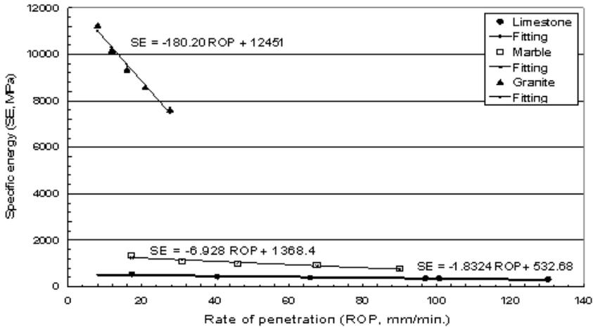
Figure (1) Relationship between average rate of penetration and specific energy for all rocks at different loads and drilling speed of 1000 rpm
