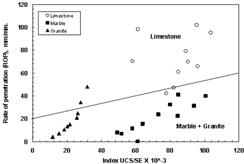
Figure (5) Relationship between UCS/SE and rate of penetration for all rocks at rotary drilling of 300 rpm and loads of 45, 60, 75, 90, 120, 150, 180, 210, 300, 390 and 480 kgf or new bit.
