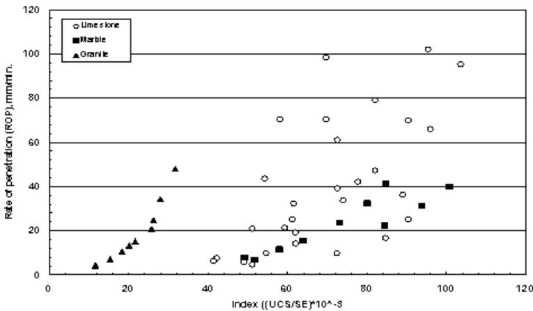
Figure (4) Relationship between UCS/SE and Rate of penetration for all rocks at different loads and rotary speed of 300 rpm with new bit.
