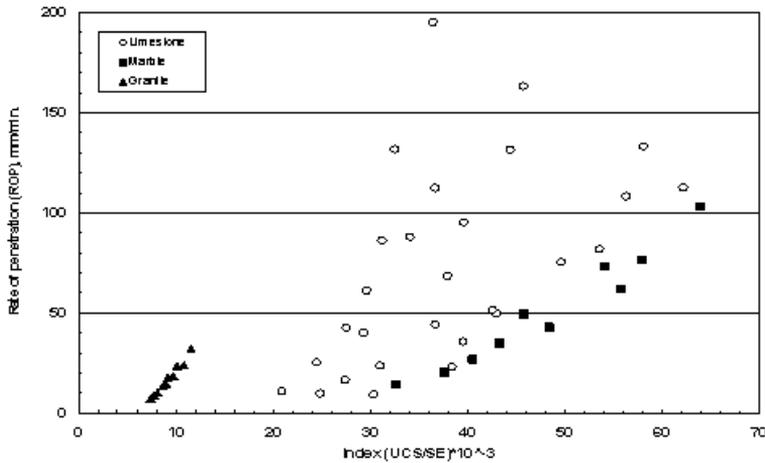
Figure (3) Relationship between UCS/SE and Rate of penetration for all rocks at different loads and rotary speed of 1000 rpm with new bit.
