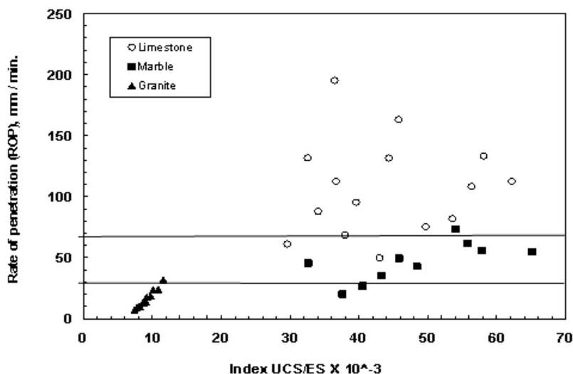
Figure (6) Relationship between UCS/SE and rate of penetration for all rocks at rotary drilling of 1000 rpm and loads of 45, 60, 75, 90, 120, 150, 180, 210, 300, 390 and 480 kg for new bit.
