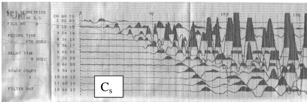
**Fig. 2: A sample of the geophone recorded seismograms for arrival times using EG&G system.**
