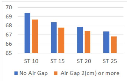
Fig. 5. Comparing Effect of Air Gap on Green Roof Performance for Deferent Soil Thickness (ST)
