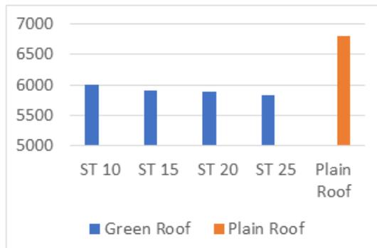
Fig. 7. Comparing Annual CO<sub>2</sub> Production (kg) of Plain Roof With Deferent Green Roof Soil Thickness (ST)
