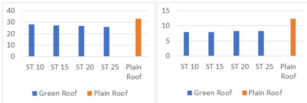
**Fig. 4.** Comparing Heating and Cooling Loads of Plain Roof and Green Roof With Different Soil Thickness (ST) (Left: Heating Load, Right: Cooling Load)
