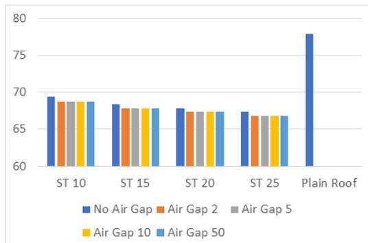
**Fig. 3.** Comparing EUJ of Green Roof Performance for Different Soil Thickness (ST) and Air Gap With Plain Roof When Apartment is Facing South
