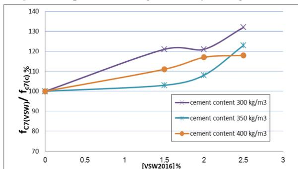
Fig. 4. Compressive strength at 28 days using (VSW2016).
