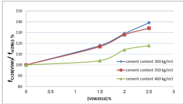
Fig. 9. Flexural of tensile strength using (VSW2016).
