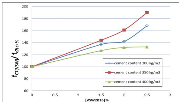
Fig. 3. Compressive strength at 7 days using (VSW2016).
