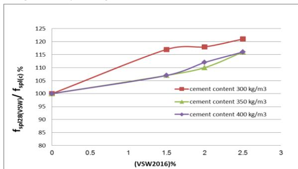
Fig. 8. Splitting tensile strength using (VSW2016).
