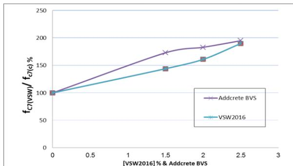
Fig. 5. Compressive strength at 7 days using BVS, (VSW2016) with C.C. 350 kg/m<sup>3</sup>.
