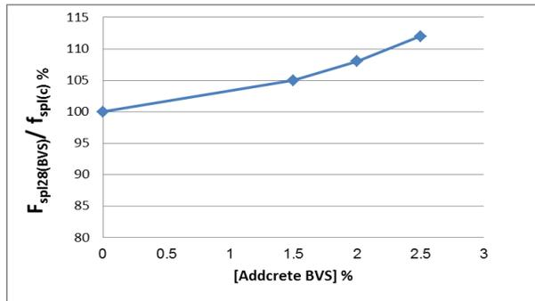
Fig. 10. Splitting tensile strength using (addcrete BVS) with (c.c) 350kg/m<sup>3</sup>
