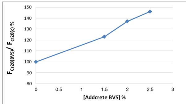
Fig. 11. Flexural of tensile strength using (addcrete BVS) with (c.c) 350 kg/m<sup>3</sup>
