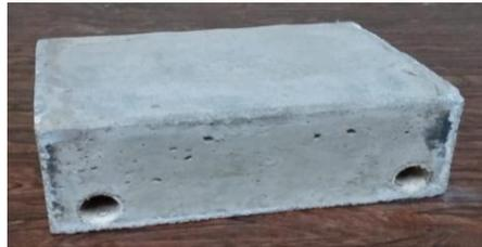
**Photo 2.** Upstream view of weir model showing bottom pipes.
