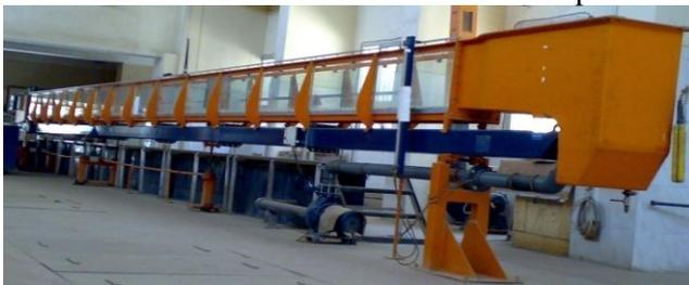
**Photo 1.** General view of the re-circulating flume.
