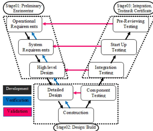
Fig.7. Life-Cycle of Interface Management process [1]
