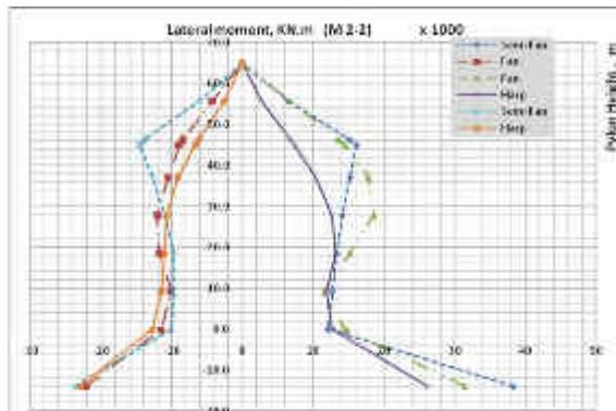
**Fig.11.** Tower lateral bending moment extreme values (beside roller support)
