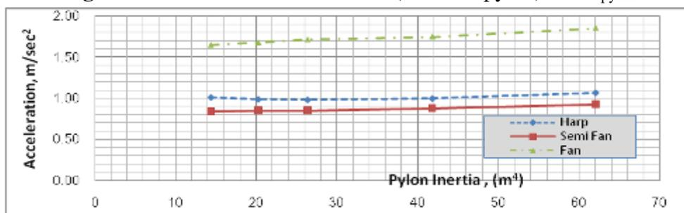
Fig. 33. The variation of acceleration at top of the pylon with  $I_{pylon}$
