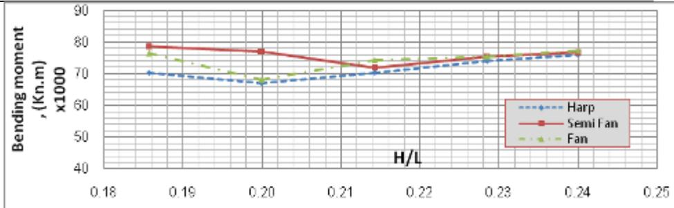
Fig. 15. The variation of the moment at the midpoint of the middle span of the deck with H/L
