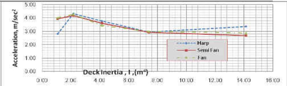
Fig. 21. The variation of the acceleration at distance 64.286m in the deck with  $I_{deck}$
