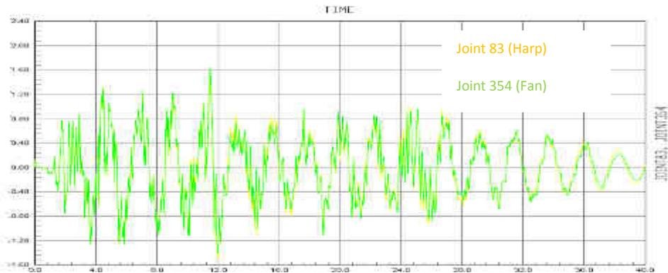
**Fig. 41.** Acceleration vs. time at the midpoint of the middle spans of the deck for harp and fan system
