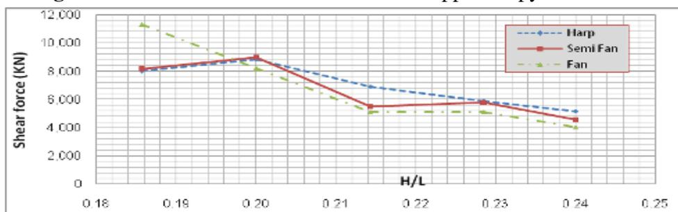
**Fig. 20.** The variation of the shear force at the support of pylon with H/L
