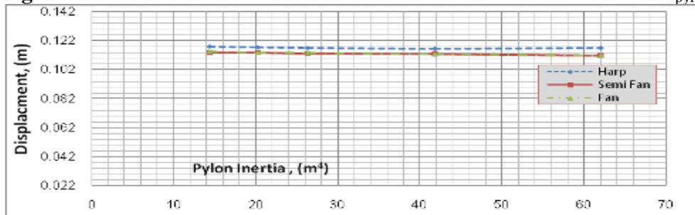
**Fig. 30.** Maximum displacement at the midpoint of the middle span of the deck with  $I_{pylon}$
