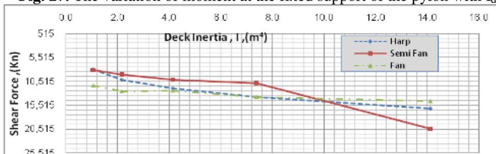
Fig. 28. The variation of shear force at the fixed support of the pylon with  $I_{deck}$
