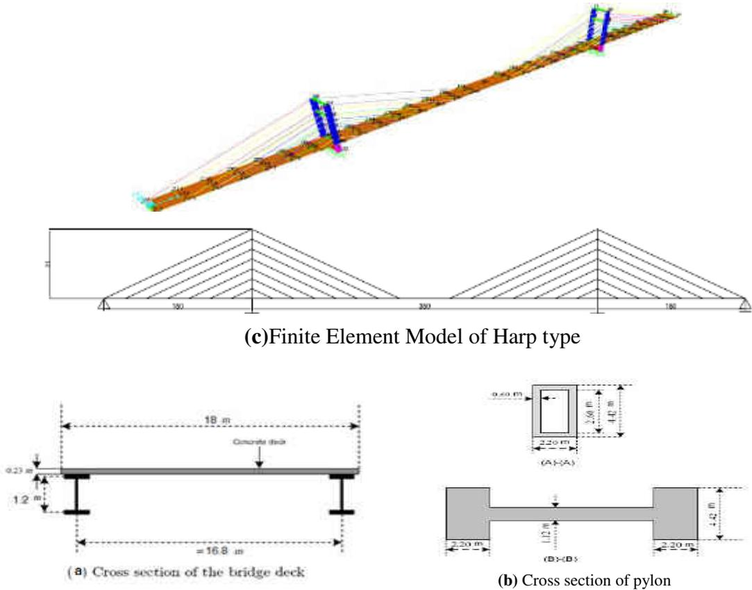
**Fig.2.** Longitudinal bridge arrangements and deck cross section
