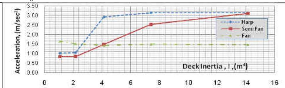
Fig. 25. The variation of acceleration at the top of the pylon with  $I_{deck}$
