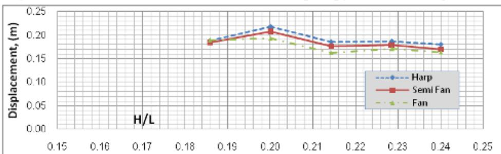
Fig. 18. The variation of the displacement at the top of pylon with change of H/L
