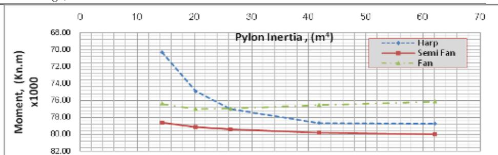
Fig. 31. Moment at the midpoint of the middle span of the deck with  $I_{pylon}$
