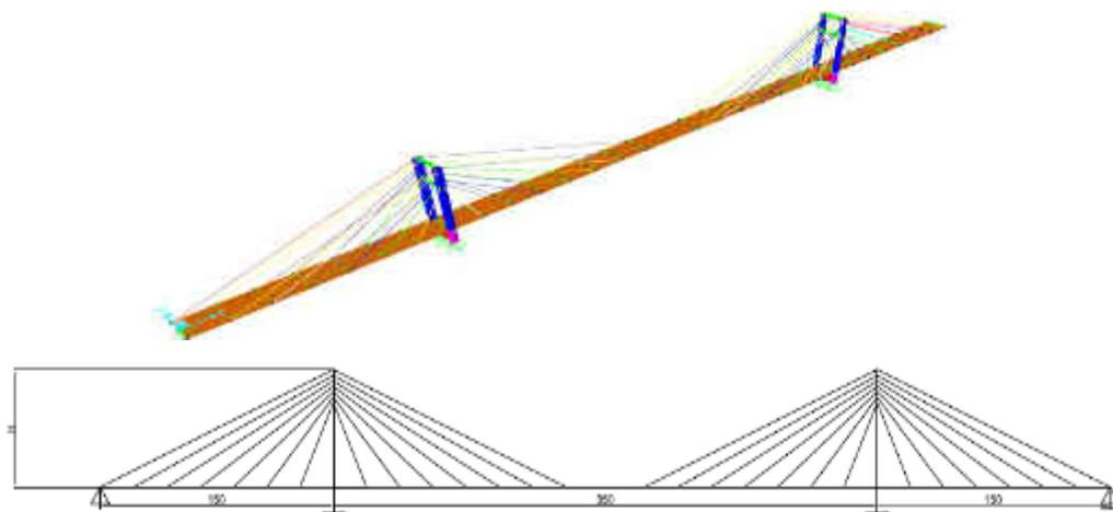
(b) Finite Element Model of Semi-Fan
