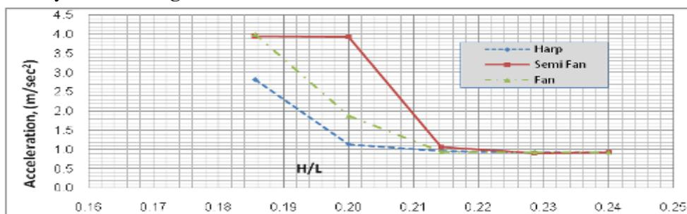
**Fig. 13.** The variation of the acceleration (at the distance 64.286m in the deck) with H/L
