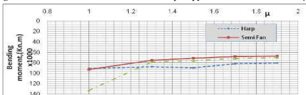
**Fig. 8.** The variation of moment at the fixed support of tower for different cases of  $\mu$
