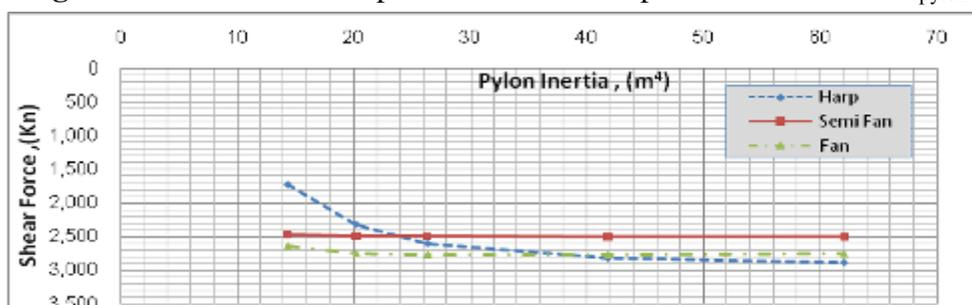
Fig. 32. The variation of shear force (Near the pylon) with  $I_{pylon}$
