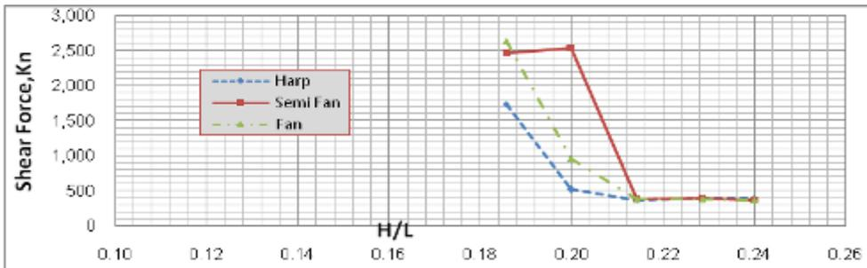
Fig. 16. The variation of the shear near the pylon with H/L
