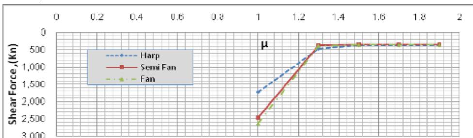
Fig. 6. The variation of the shear force on the deck (Near the pylon) with μ
