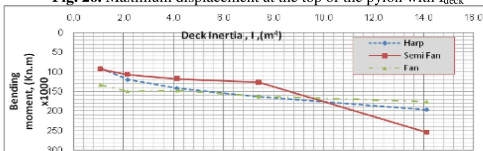
Fig. 27. The variation of moment at the fixed support of the pylon with  $I_{deck}$
