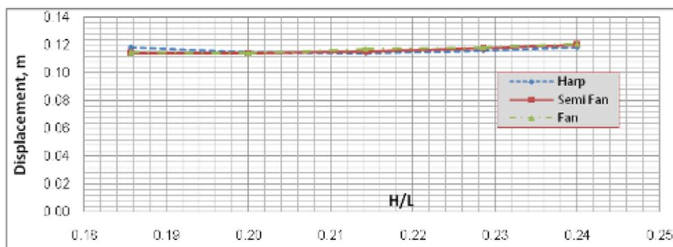
**Fig. 14.** The variation of the displacement at the midpoint of the middle span of the deck with H/L
