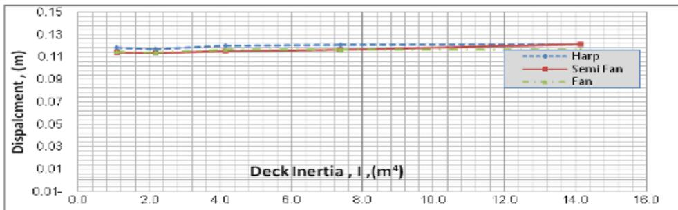
Fig. 22. Maximum displacement at the midpoint of the middle span of the deck with  $I_{deck}$
