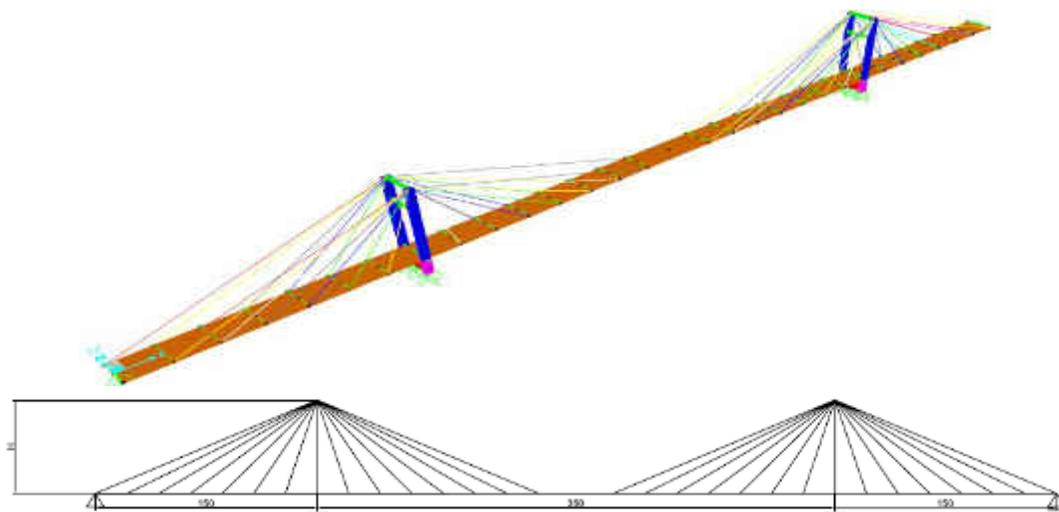
(a) Finite Element Model of Fan type
