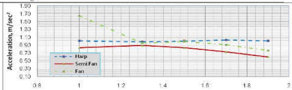
**Fig. 7.** The variation of acceleration at the top of pylon for different cases of  $\mu$
