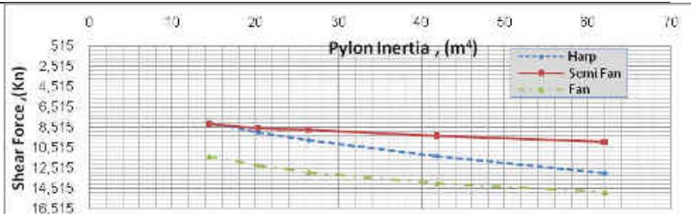
**Fig. 35.** The variation of shear force at fixed support of the pylon with  $I_{\text{pylon}}$
