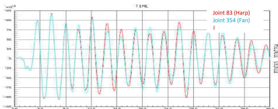
**Fig. 43.** Displacement vs. time at the midpoint of the middle spans of the deck for harp and fan system
