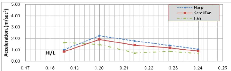
Fig. 17. The variation of acceleration at the top of pylon with change of H/L
