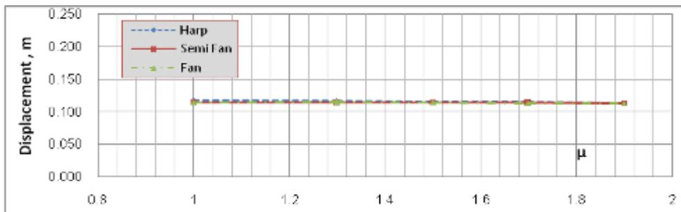
Fig. 4. The variation of the maximum displacement at the midpoint of the middle span of the deck with μ
