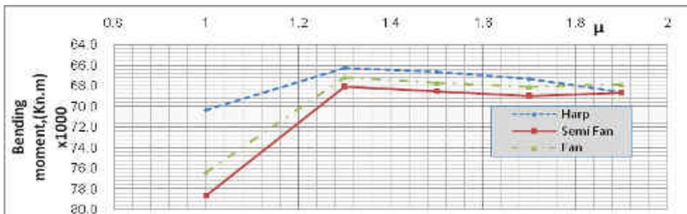
Fig. 5. The variation of the moment at the midpoint of the middle span of the deck with μ
