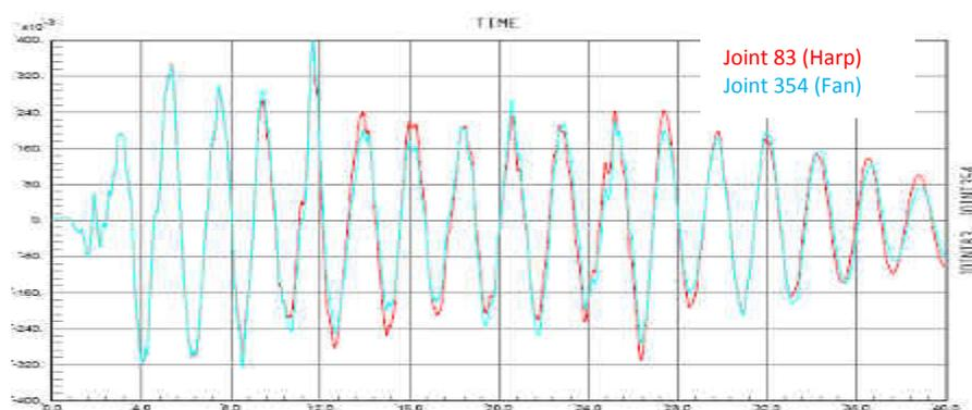
**Fig. 42.** Velocity vs. time at the midpoint of the middle spans of the deck for harp and fan system
