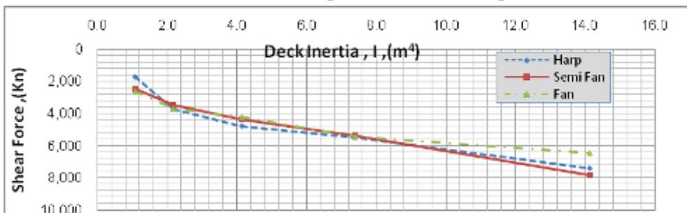
Fig.24. The variation of shear force at a distance near the pylon with  $I_{deck}$
