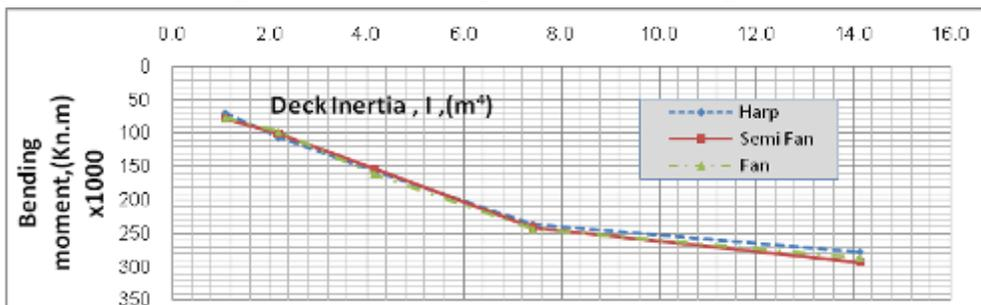
Fig. 23. The variation of moment at the midpoint of the middle span of the deck with  $I_{deck}$
