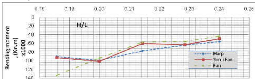
**Fig. 19.** The variation of the moment at the support of pylon with H/L
