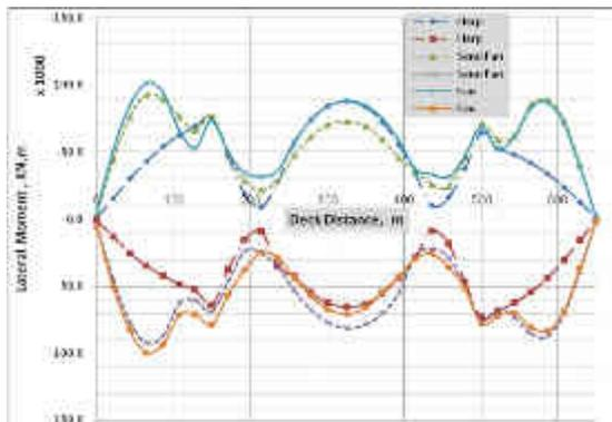
**Fig.12.** Deck lateral bending moment extreme values
