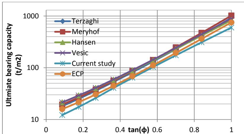
**Fig. 12.** Ultimate bearing capacity versus  $\tan \phi$  at  $B = 1.0$  m,  $R_f = 1$ ,  $c = 2$   $t/m^2$  using different methods
