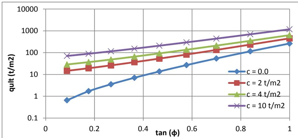
Fig. 5. Ultimate bearing pressure versus tan φ at R<sub>f</sub> = 0.0 for different values of c
