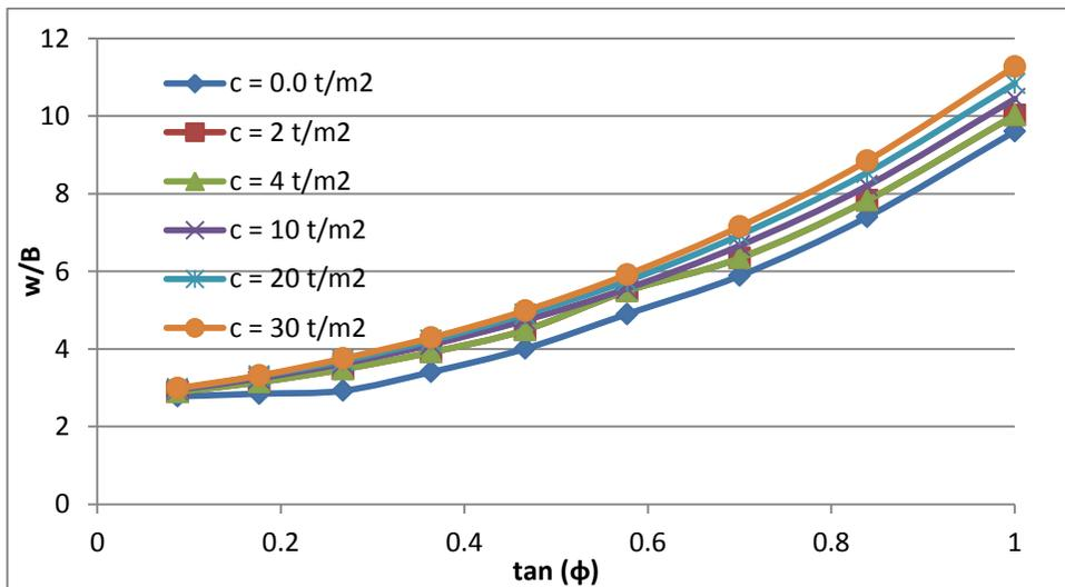
**Fig. 10.** Maximum extent of failure surface ( $w/B$ ) versus  $\tan(\phi)$  at  $R_f = 0.0$  and  $B = 2 \text{ m}$  for different values of  $c$
