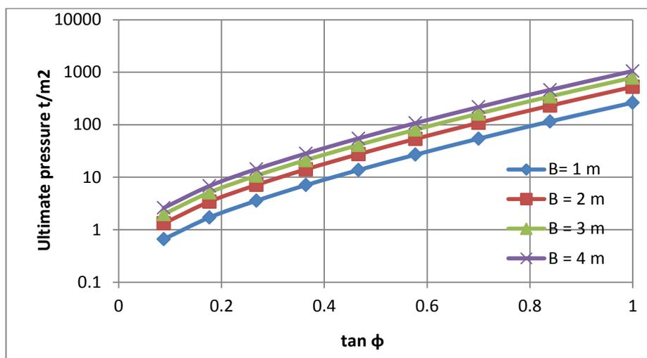
**Fig. 3.** Ultimate bearing capacity versus  $\tan \phi$  at  $R_f = 0.0$  for different values of  $B$
