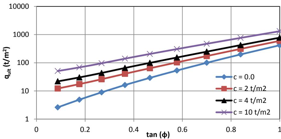
Fig. 6. Ultimate bearing capacity versus tan φ at R<sub>f</sub> = 1 for different values of c
