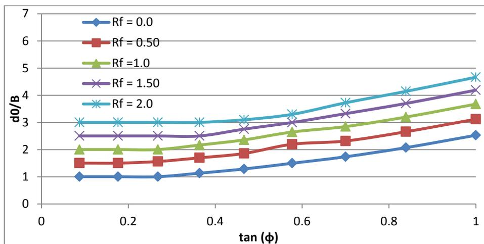
**Fig. 8.** Maximum depth of failure surface ( $d_0/B$ ) versus  $\tan(\phi)$  at  $c = 0.0$  for different values of  $R_f$
