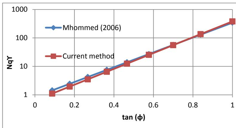
**Fig. 13.** Bearing capacity factor ( $N_{q\gamma}$ ) versus  $\tan \phi$  at  $R_f = 0.0$  for Mohammed [15] and current method s
