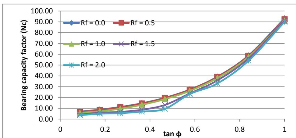
**Fig. 11.** Bearing capacity factor ( $N_c$ ) versus  $\tan \phi$  for different  $R_f$
