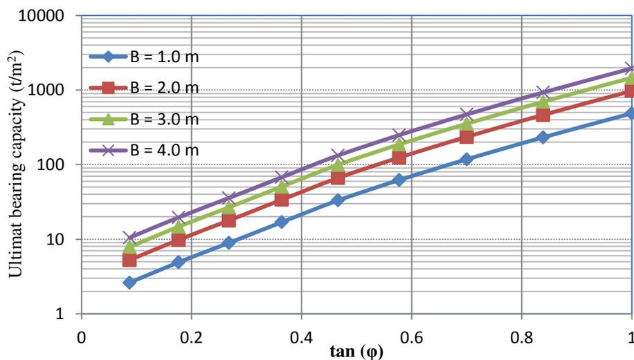
**Fig. 4 .** Ultimate bearing capacity versus  $\tan \phi$  at  $R_f = 1.5$  for different values of  $B$
