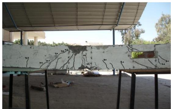
Plate (11): The pattern of cracks and mode of failure of beam (B11)
