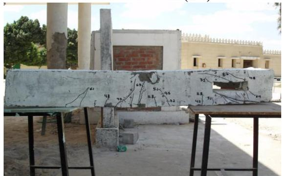
Plate (5): The pattern of cracks and mode of failure of beam (B5)
