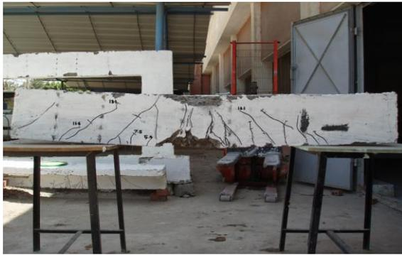
Plate (1): The pattern of cracks and mode of failure of beam (B1)
