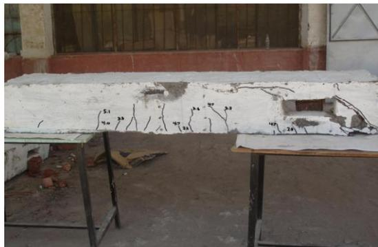
Plate (9): The pattern of cracks and mode of failure of beam (B9)
