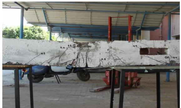
Plate (6): The pattern of cracks and mode of failure of beam (B6)
