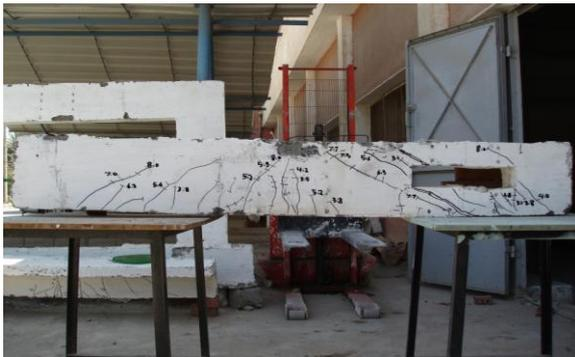
Plate (8): The pattern of cracks and mode of failure of beam (B8)
