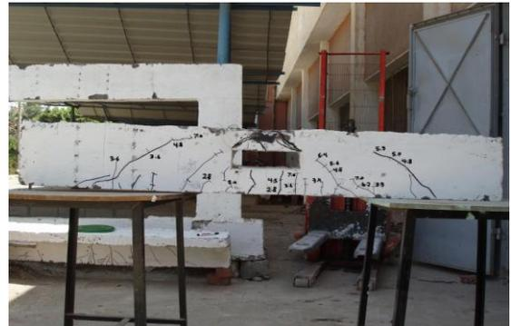
Plate (4): The pattern of cracks and mode of failure of beam (B4)
