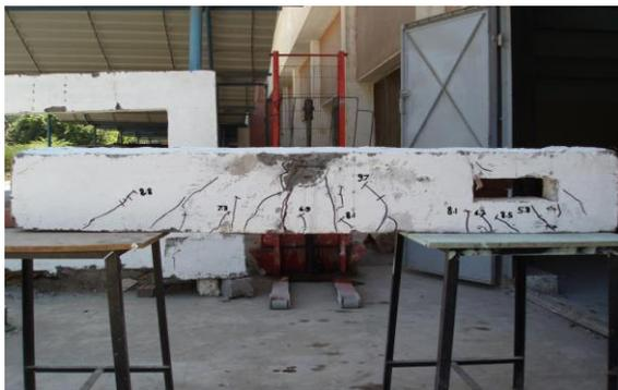
Plate (2): The pattern of cracks and mode of failure of beam (B2)
