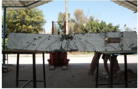
Plate (10): The pattern of cracks and mode of failure of beam (B10)
