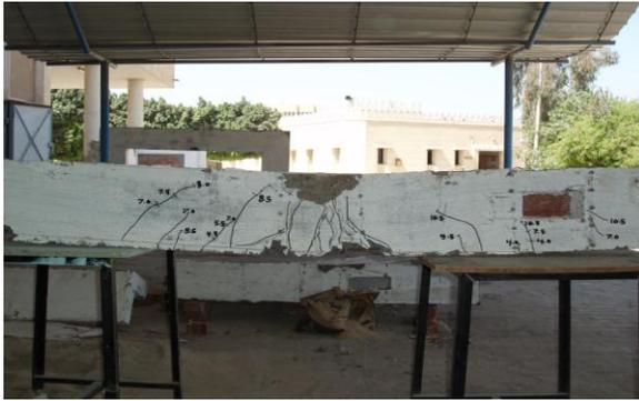
Plate (7): The pattern of cracks and mode of failure of beam (B7)
