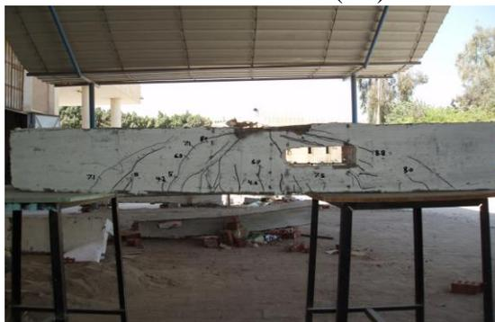
Plate (3): The pattern of cracks and mode of failure of beam (B3)
