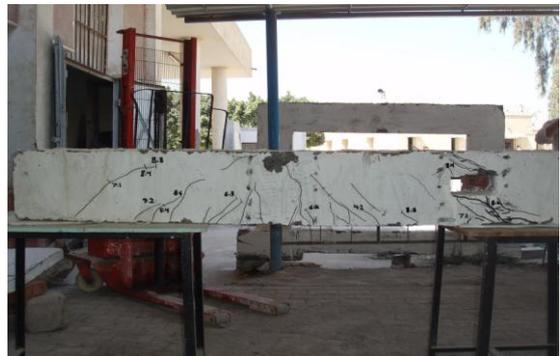
Plate (12): The pattern of cracks and mode of failure of beam (B12)
