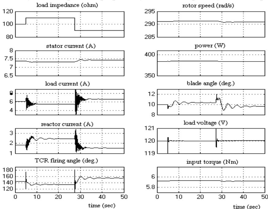
Fig. (6): Dynamic response of proposed system with step change in load impedance.
