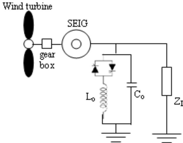
Fig.(1): Schematic representation of the wind energy system
