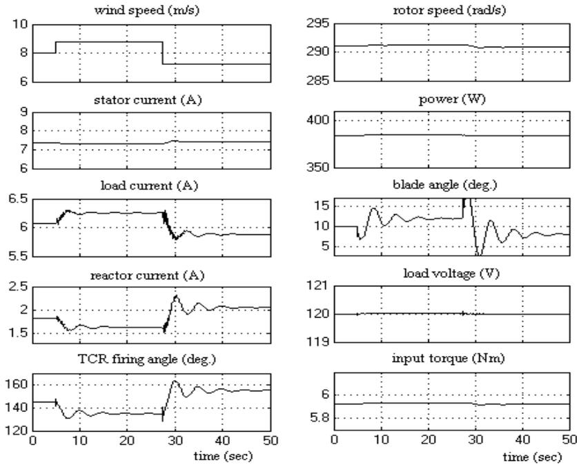
Fig. (7): Dynamic response of the proposed system with a step change in wind speed and parameters changes.
