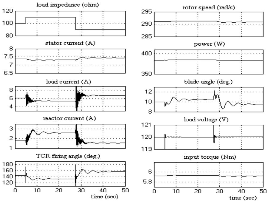
Fig. (8): Dynamic response of the proposed system with a step change in load impedance and parameters changes.
