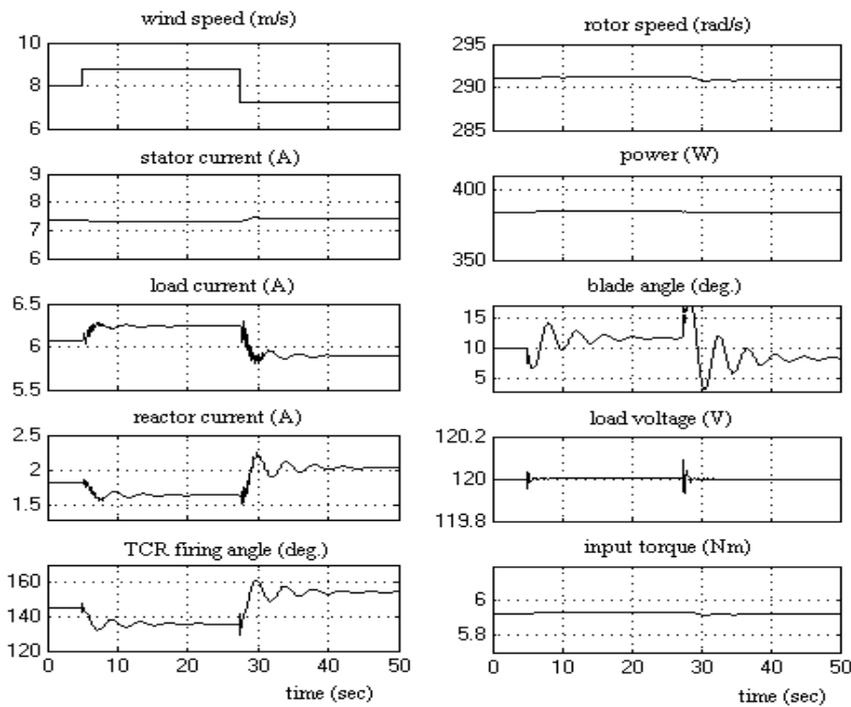
Fig. (5): Dynamic response of proposed system with step change in wind speed.
