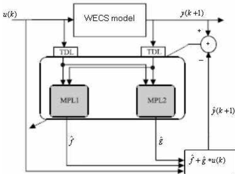
Fig. 2: NARMA-L2 plant model identification
