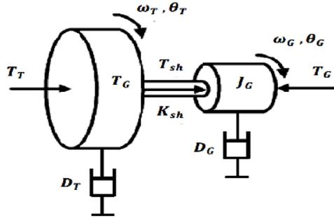
Fig. (1) Two mass drive train model of wind turbine
