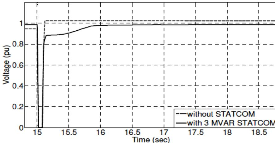
Fig. (13) The voltage of bus B25 during three-phase to ground fault.
