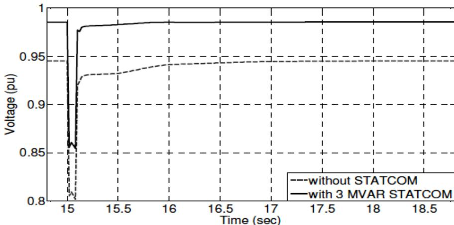
Fig. (7) The voltage of bus B25 during single phase to ground fault.
