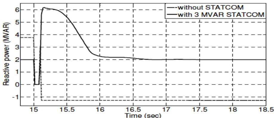
Fig. (15) The reactive power at bus B25 during three-phase to ground fault.
