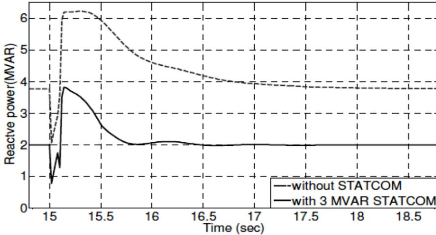
Fig. (12) The reactive power at bus B25 during double phase to ground fault.
