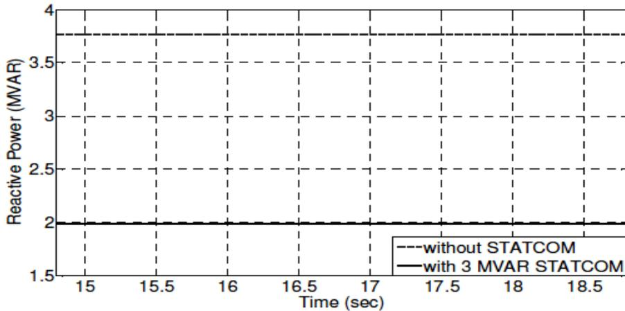
Fig. (4) The reactive power at bus B25 during steady state operation.
