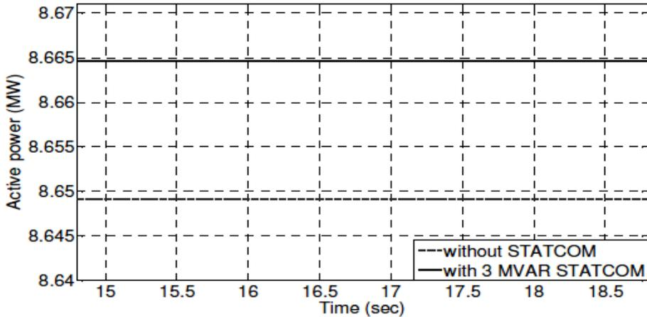
Fig. (6) The active power at bus B25 during steady state operation.
