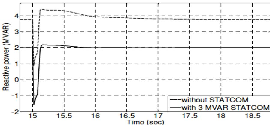
Fig. (9) The reactive power at bus B25 during single phase to ground fault.
