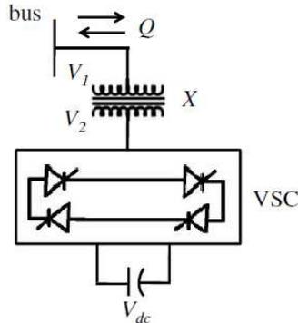
Fig. (2) A controllable voltage source VSC.
