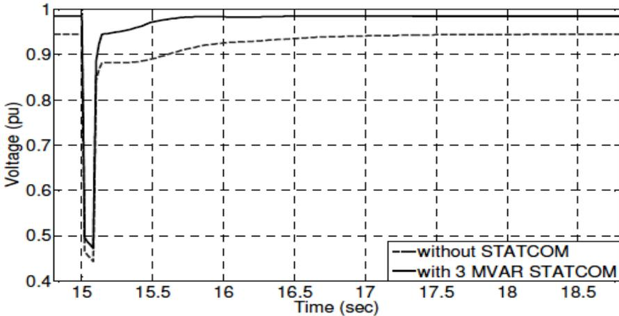
Fig. (10) The voltage of bus B25 during double phase to ground fault.
