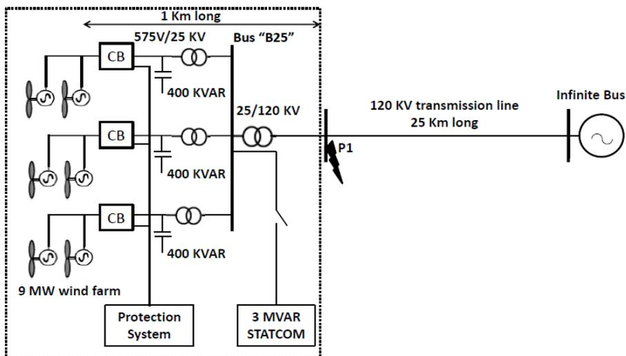
Fig. (3) Single line diagram of the studied system.
