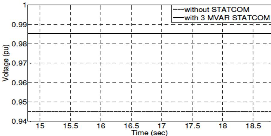
Fig. (5) The voltage of bus B25 during steady state operation.
