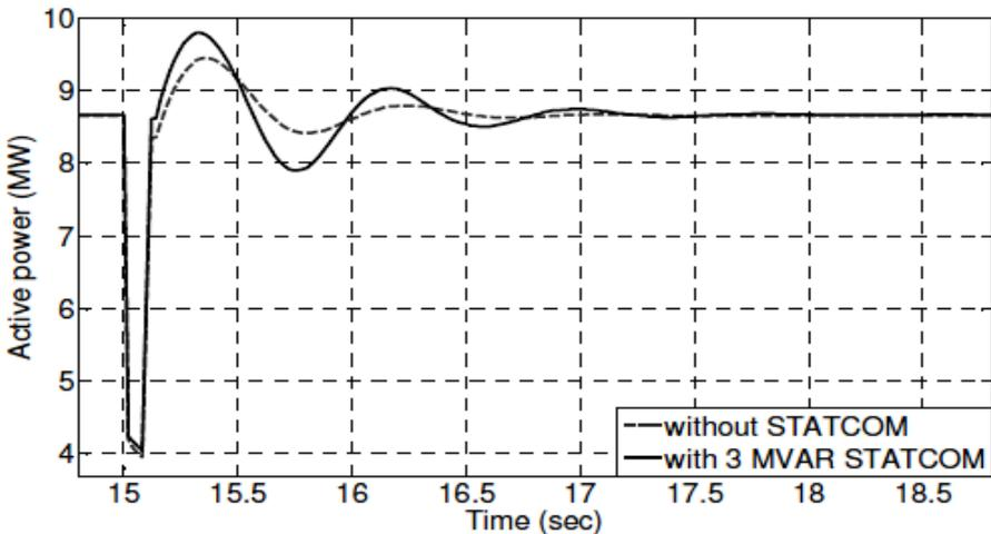
Fig. (11) The active power at bus B25 during double phase to ground fault.
