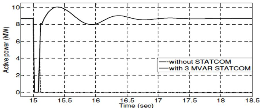
Fig. (14) The active power at bus B25 during three-phase to ground fault.
