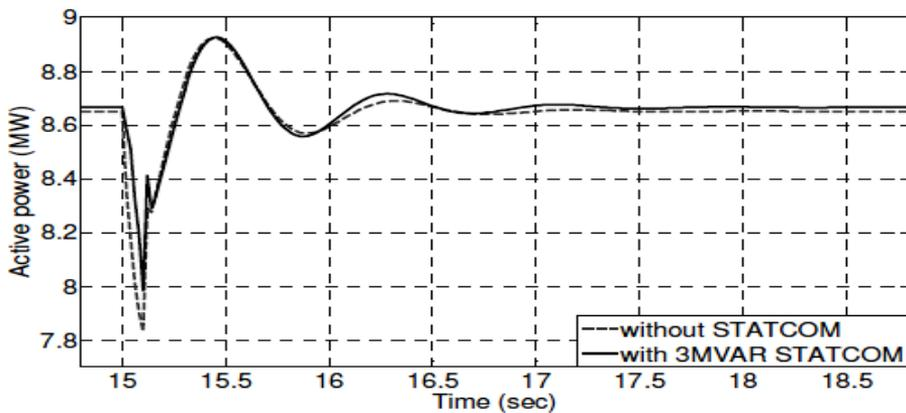
Fig. (8) The active power at bus B25 during single phase to ground fault.
