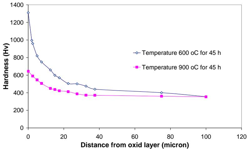
**Figure 7.** Microhardness-depth profiles for oxidised Ti-6Al-4V samples treated at 600°C and 900°C for 45 h.
