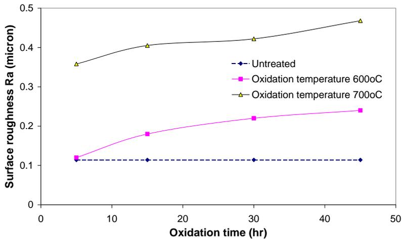
**Figure 2.** Effect of oxidation temperature and oxidation time on the roughness of oxidation surface.
