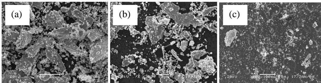
**Figure 11.** Wear debris of thermally oxidised samples tested at 1 m/s sliding velocity, 100 N applied load, and 3000 m sliding distance a) treated at 600 °C for 45 h, b) treated at 700 °C for 45 h, and c) treated at 900 °C for 45 h.
