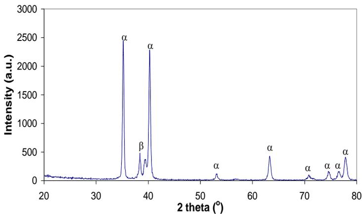
**Figure 3.** XRD pattern of untreated sample ( $\alpha$ : hcp titanium,  $\beta$ : bcc titanium).
