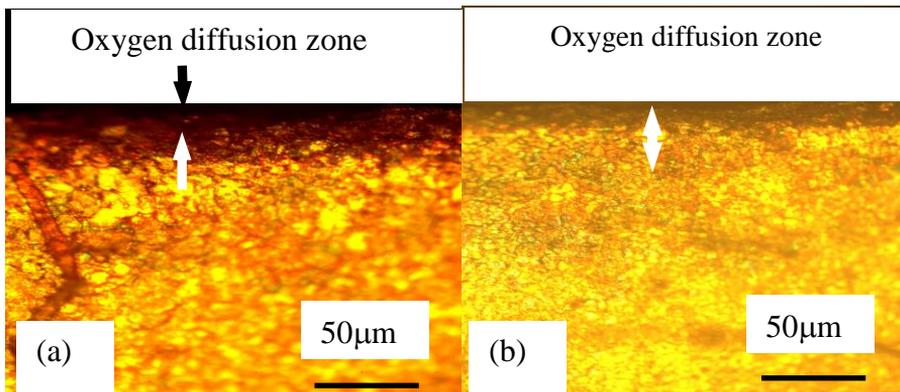
**Figure 6.** Cross-sectional optical micrographs of a sample oxidized at a) 600 °C for 45 h, and b) 900 °C for 45 h.
