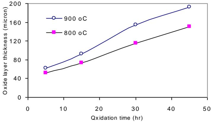
**Figure 1.** Effect of oxidation time on the thickness of oxide layer at high temperature.
