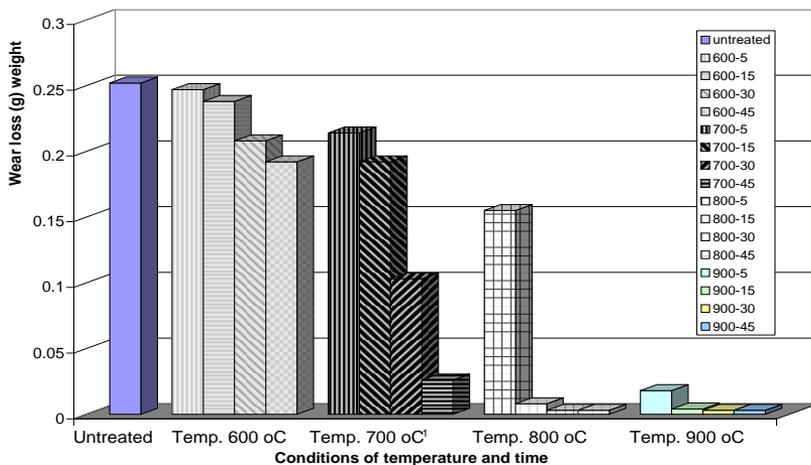
**Figure 8.** Wear loss vs. treatment conditions of untreated and thermally oxidised samples tested with 100 N coupling load, 1 m/s sliding velocity and 3000 m sliding distance.
