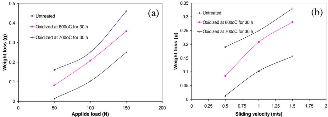
**Figure 9.** Wear weight loss of untreated and treated samples at 600 °C and 700 °C for 30 h at constant sliding distance (3000 m) versus a) applied load, and b) sliding velocity.
