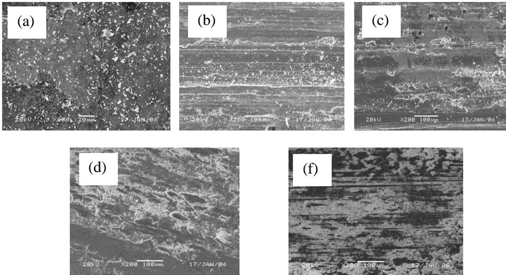
**Figure 10.** SEM micrographs of a) surface of oxidised sample at 800 °C for 45 h, b) wear tracks of sample treated at 600 °C for 45 h, c) wear tracks of sample treated at 700 °C for 45 h, d) wear tracks of sample treated at 800 °C for 45 h, and e) wear tracks of sample treated at 900 °C for 45 h.
