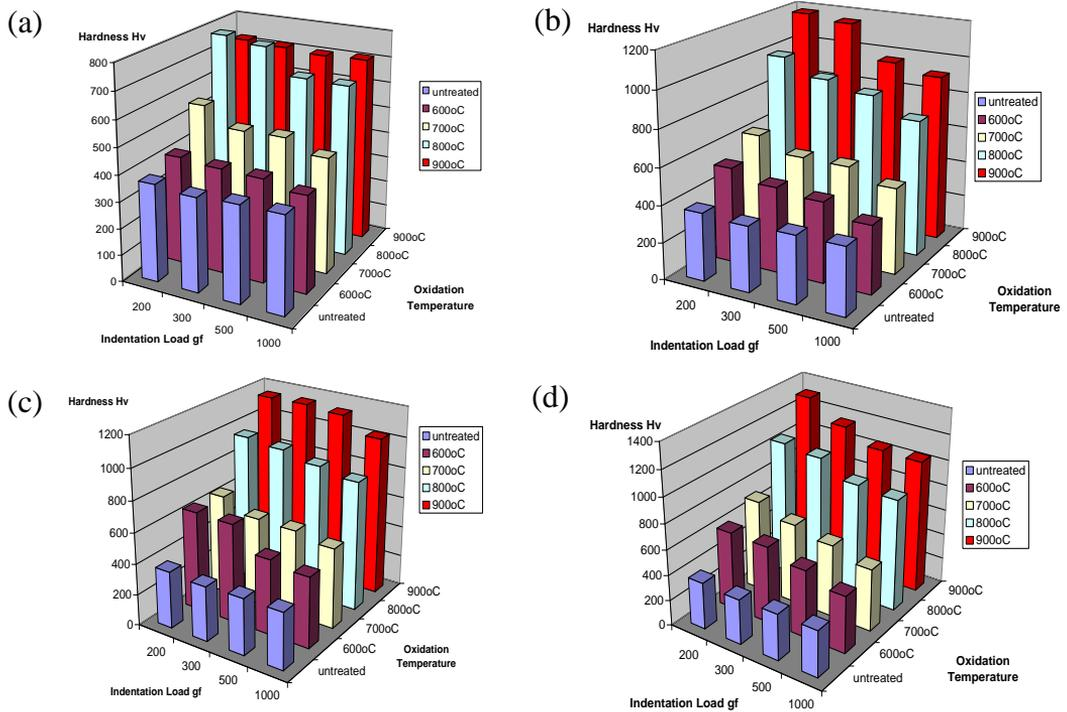
**Figure 5.** Effect of oxidation time on the hardness of samples a) 5 hr, b) 15 hr, c) 30 hr, and d) 45 hr.
