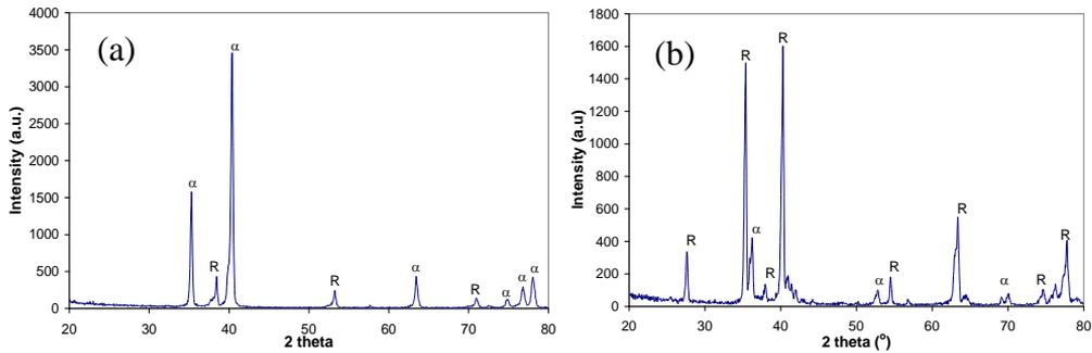
**Figure 4.** XRD patterns for oxidized samples a) after oxidation at 600°C for 30 h, and b) after oxidation at 800°C for 30 h.
