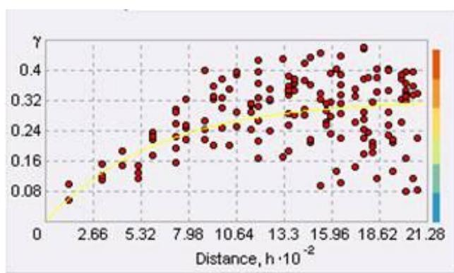
**Figure 5:** The semivariogram and fitted model for P<sub>2</sub>O<sub>5</sub> %.
