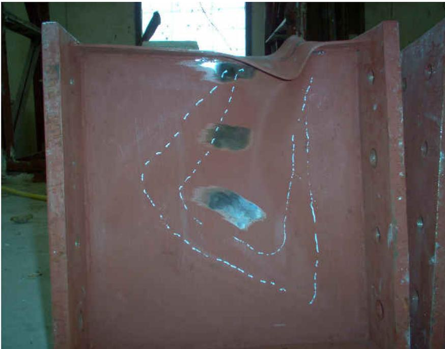
**Fig. 4d:** N.C.F. F.W. specimen after failure.
