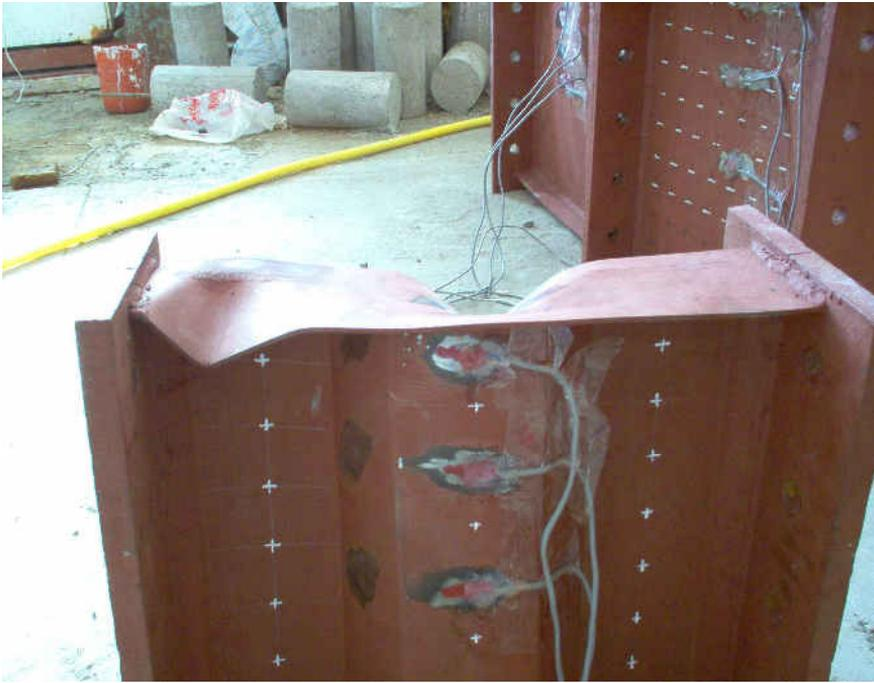
**Fig. 4c:** N.C.F. C.W. specimen after failure.
