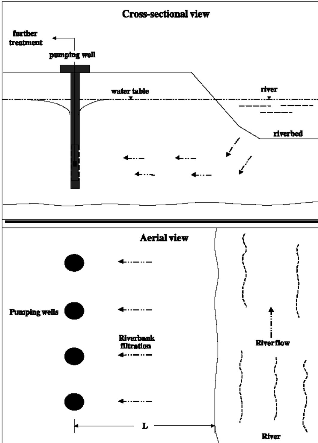
Fig. 1: Schematic drawing of riverbank filtration [10].
