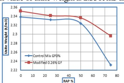
Fig. 12. Relationship between unit weight and RAP % at 0.26% (GF)
