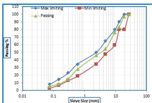
**Fig. 3.** Adopted gradation of aggregate used
