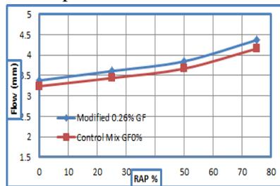
Fig. 15. Relationship between Flow and RAP % at 0.26% (GF)
