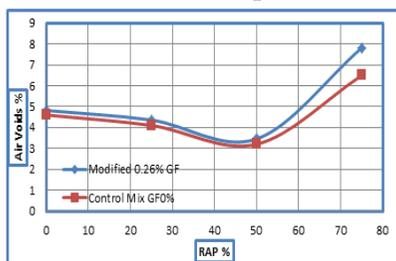
Fig. 14. Relationship between Air Voids and RAP % at 0.26% (GF)
