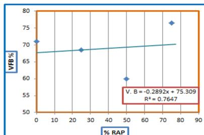
Fig. 11. Effect of Increasing RAP% on VFB
