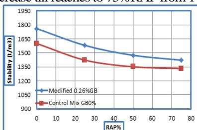
Fig. 13. Relationship between Stability and RAP % at 0.26% (GF)
