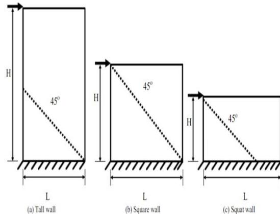
Fig.6. Direction of diagonal cracks in masonry shear walls [38].
