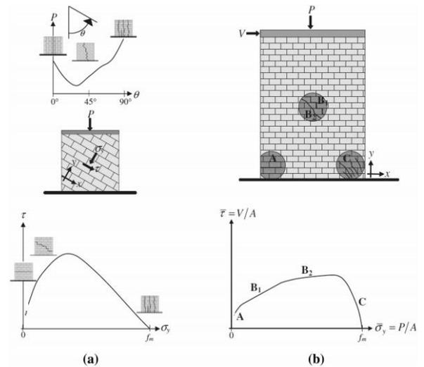
Fig.7. Failure modes and limit domains for masonry: a) Scale of the material; b) Scale of the pier from [41].
