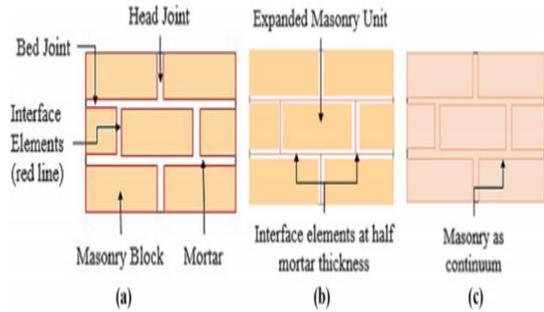
Fig.8. Modeling strategies of masonry structures: a) detailed micro-modeling; b) simplified micro-modeling; and c) macro-modeling [51].
