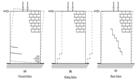
Fig.1.The failure modes of masonry wall [23].
