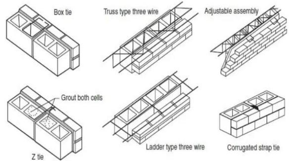
Fig.3. Joint Reinforcement Applications in Masonry
