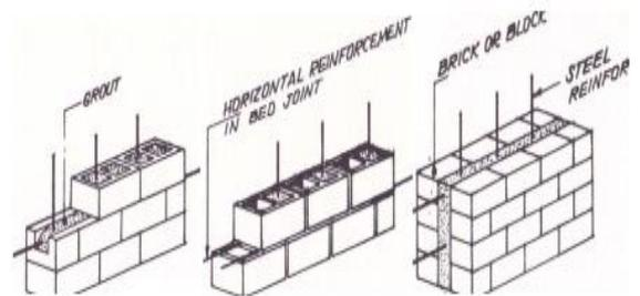
Fig.4. Placing of reinforcement in masonry
