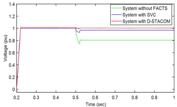
Fig. 9. The voltage magnitude during a sudden heavy load with and without D-FACTS.
