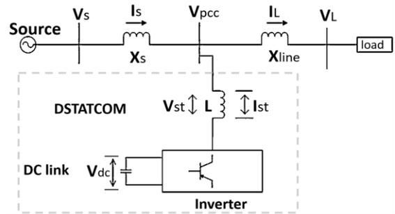
Fig.2. D-STATCOM with the electrical power system.
