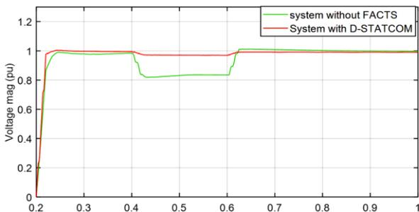
Fig. 6. Single-line to ground voltage magnitude with and without D-STATCOM.
