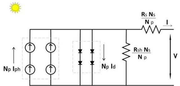
Fig.5. The equivalent circuit of PV array.
