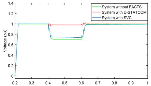
Fig. 7. Double line - ground voltage magnitude with and without D-FACTS.
