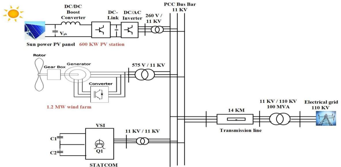
Fig.3. proposed Grid with PV/wind hybrid power system and D-STATCOM.
