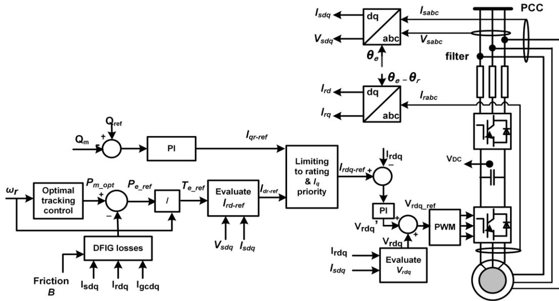
Fig.4. Control scheme of rotor side converter.
