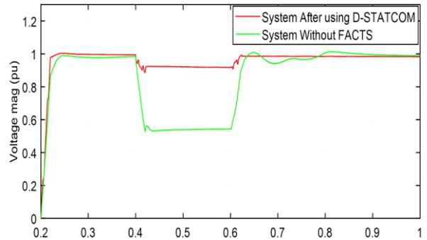
Fig.8. Three phase - ground voltage magnitude with and without D-STATCOM.
