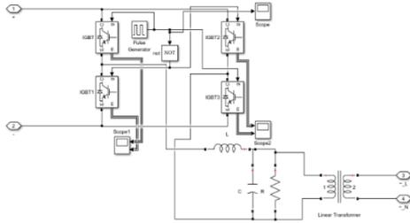
Fig.6. Block diagram of the inverter
