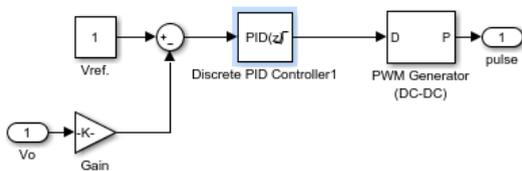
Fig.10. PID control circuit.
