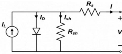
Fig.3.The electrical equivalent circuit of a solar cell.
