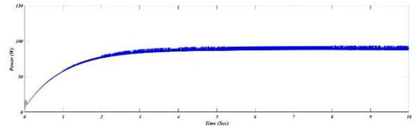
Fig.18.The simulated output power of the fuel cell system as a function of time variation.
