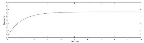
Fig.19.The simulated output current of the fuel cell system as a function of time variation.
