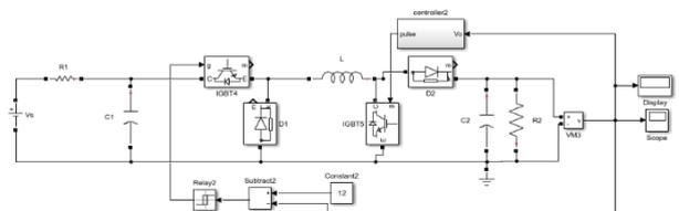
Fig.12. Buck-Boost converter equivalent circuit.
