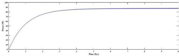
Fig.13.The simulated output power of the wave energy conversion system as a function of time variation
