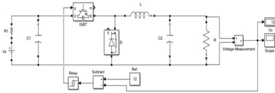
Fig.9. Buck converter circuit.
