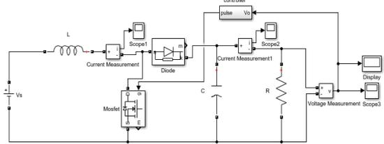
Fig.11. Boost converter circuit.
