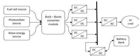
Fig.1.The block diagram of the integration system
