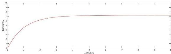
Fig.15.The simulated output current of the wave energy conversion system as a function of time variation
