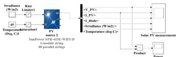
Fig. 4. Solar PV model in Matlab/Simulink.
