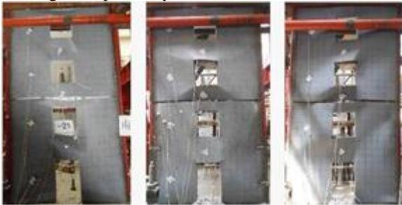
Fig. 4. An example of Strengthening coupled shear walls by external steel plates [32].
