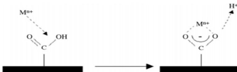
Fig. (4) Cation exchange mechanism with the carbon surface carboxylic group[19]
