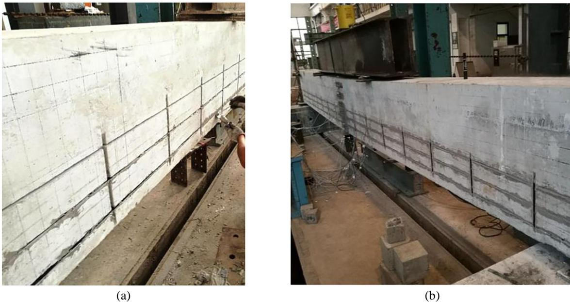
Fig. 19: Test setup and strengthening locations; (a) Mounted CFRP and filled epoxy in the groove and (b) Test load [41].
