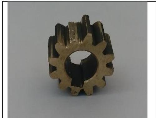
Fig. 2 Missing one tooth
