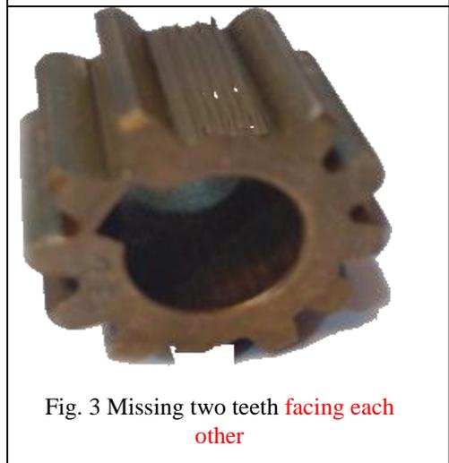
Fig. 3 Missing two teeth facing each other
