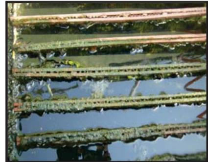
Figure 8: Growth of biomass on the media used for the IFAS system
