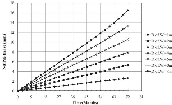
Fig. (4): Effect of Depth of Wetting on Net Pile Heave.
