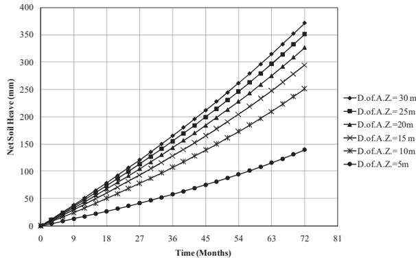
**Fig. (8): Effect of Depth of Active Zone on Soil Heave.**
