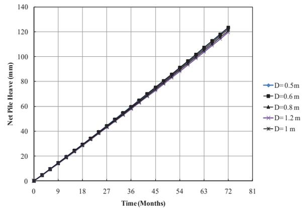
Fig. (14): Effect of Pile Diameter on Pile Heave (Piles Embedded in Expansive Clay).
