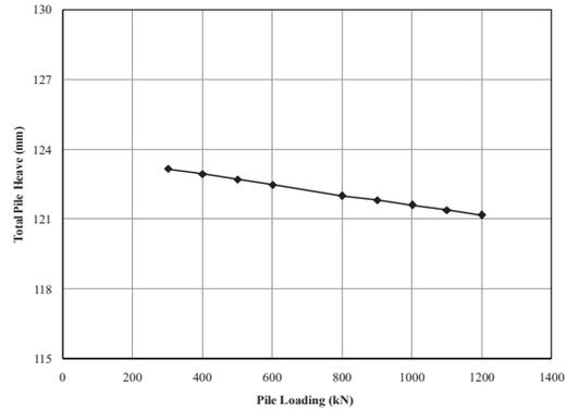
**Fig. (18): Total Pile Heave for Different Pile Loading (Piles embedded in Expansive Clay).**
