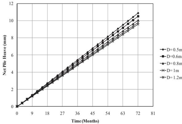
Fig. (12): Effect of Pile Diameter on Pile Heave (Piles Embedded in Sand).
