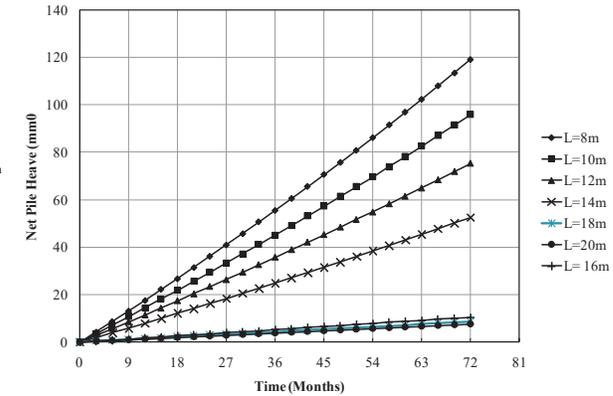
**Fig. (10): Effect of Pile Length on Net Pile Heave**
