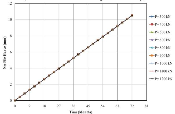
Fig. (15): Effect of Pile Loading on Pile Heave (Piles embedded in Sand).
