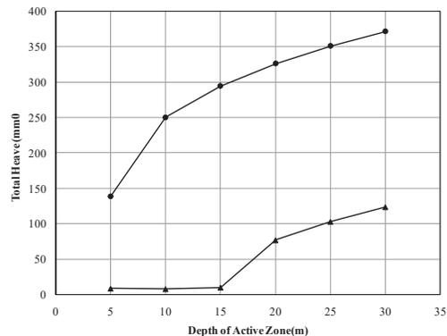
**Fig. (9): Total Pile and Free Field Heave for Different Depths of Active Zone.**
