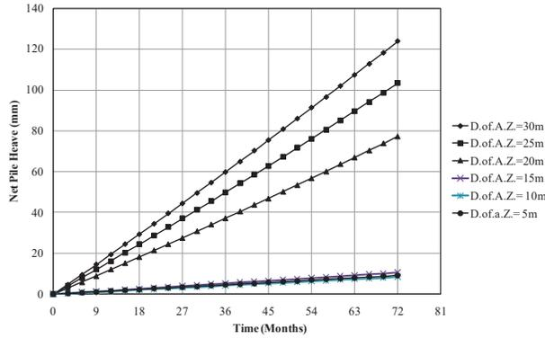
**Fig. (7): Effect of Depth of Active Zone on Pile Heave.**
