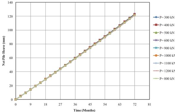
**Fig. (17): Effect of Pile Loading on Pile Heave (Piles in Uniform Expansive Clay).**
