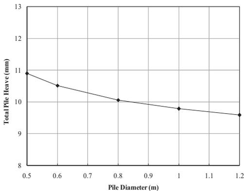
Fig. (13): Total Pile Heave for Different Pile Diameters (Piles Embedded in Sand).
