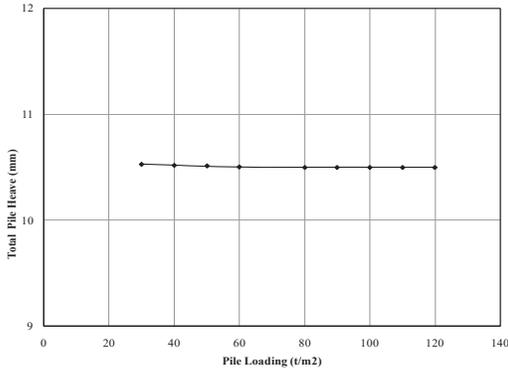
**Fig. (16): Total Pile Heave for Different Pile Loading (Piles embedded in Sand).**
