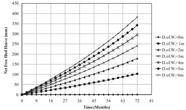
Fig. (5): Effect of Depth of Wetting on Free Field Heave.
