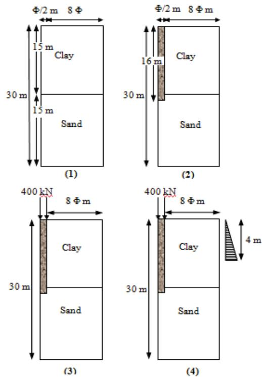
**Fig. (2): Schematic Sequence of Soil and Pile Loading.**
