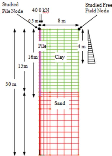
**Fig. (1): Finite Element Mesh for the Proposed Numerical Model.**
