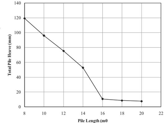
**Fig. (11): Total Pile Heave for Different Pile Lengths.**
