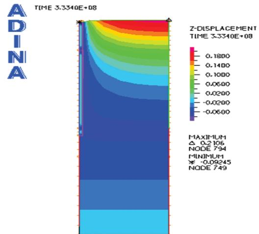
**Fig. (3): Heave Plot for 8-m Pile Length and 4-m Depth of Wetting.**
