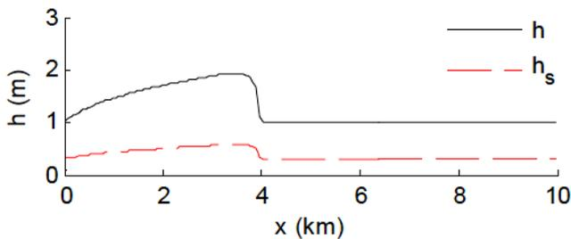
**Fig. 2. Water depth  $h$  and sediment depth  $h_s$  at  $t=1000$  s.**
