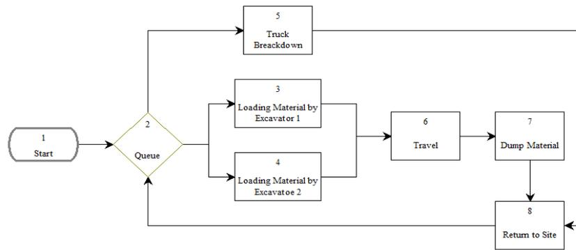
Fig. 5. Simulation model of excavation operation (case 2)
