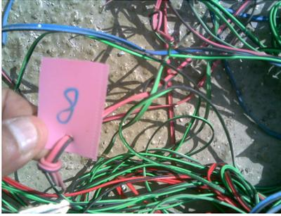
Fig.(21a): Strain gauges numbering
