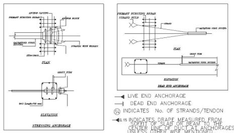
Fig.(5): Dead and live ends of tendon
