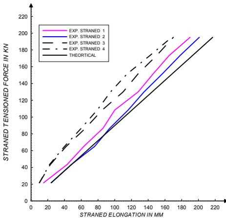
FIG.(4.1c) EXPERIMENTAL & THEORTICAL ELONGATION OF TENDON 3
