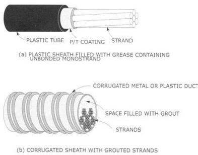
**Fig. (1): Illustration of bonded and unbonded systems (11)**
