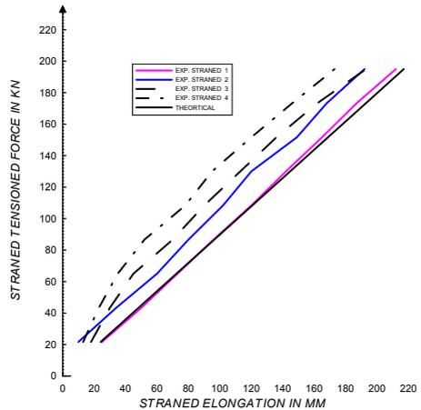
FIG.(4.1e) EXPERIMENTAL & THEORTICAL ELONGATION OF TENDON 5
