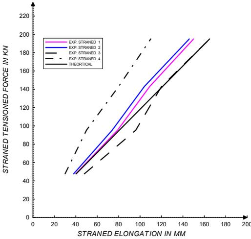
FIG.(4.2a) EXPERIMENTAL & THEORETICAL ELONGATION OF TENDON 6
