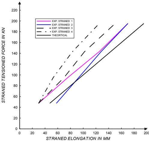
FIG.(4.2b) EXPERIMENTAL & THEORETICAL ELONGATION OF TENDON 7
