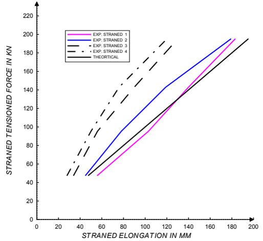
FIG.(4.2c) EXPERIMENTAL & THEORETICAL ELONGATION OF TENDON 8
