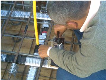
**Fig.(20a): Strain gauges at interior column**
