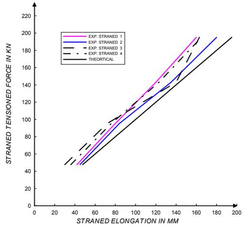
FIG.(4.2d) EXPERIMENTAL & THEORETICAL ELONGATION OF TENDON 9
