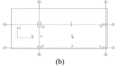
**Fig. (28): Strain gauges for studied connections at top and bottom of slab, in both directions from points 1 to 8**
