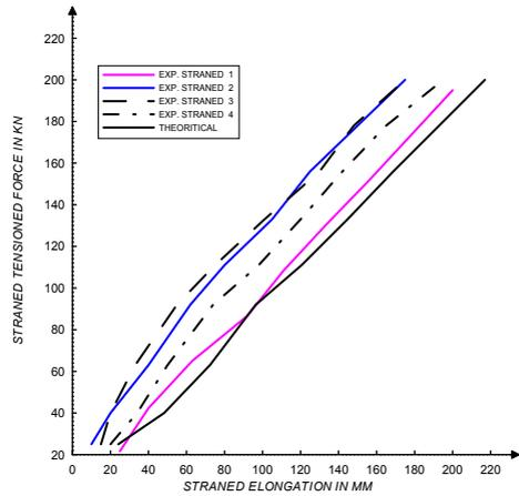
FIG.(4.1d) EXPERIMENTAL & THEORTICAL ELONGATION OF TENDON 4
