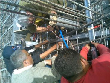
**Fig. (20b): Strain gauges at interior column**
