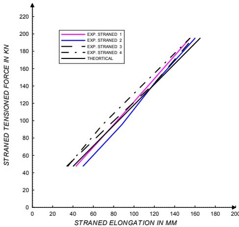
FIG.(4.2e)0 EXPERIMENTAL &amp; THEORETICAL ELONGATION OF TENDON 10
