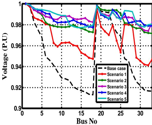
Fig. 6. Bus voltage profile of 33-bus network
