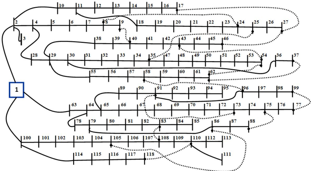
Fig. 5.118-node RDN (tie is represented by dotted line)
