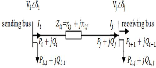
Fig. 1. Section of RDN of the  $ij$  bus
