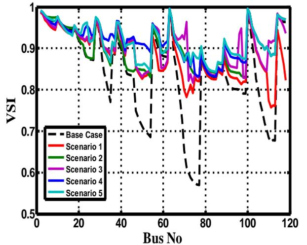
Fig. 9. Bus VSI profile of 118-bus network
