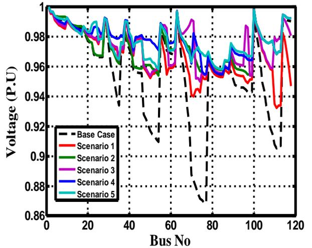
Fig. 8. Bus voltage profile of 118-bus network
