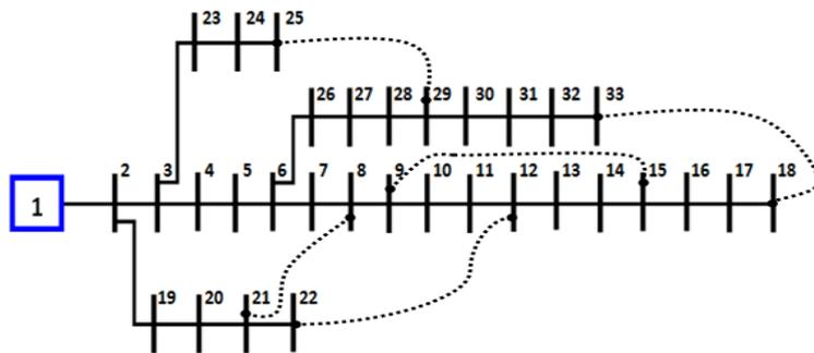
Fig. 4.33-node RDN (tie is represented by dotted line)
