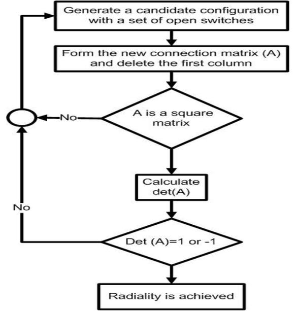
Fig. 2. Procedures to check system radiality
