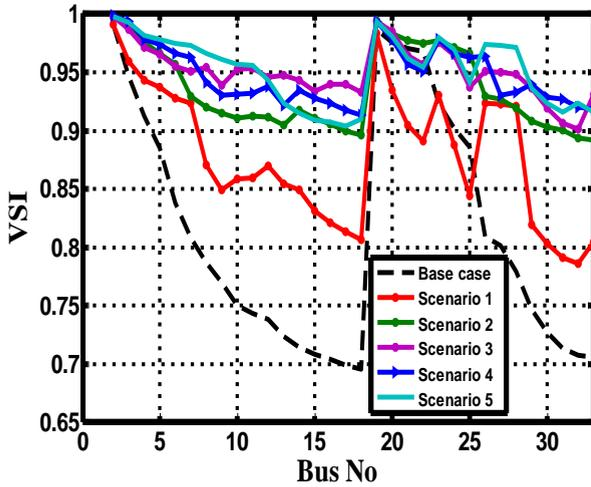
Fig. 7. Bus VSI profile of 33-bus network
