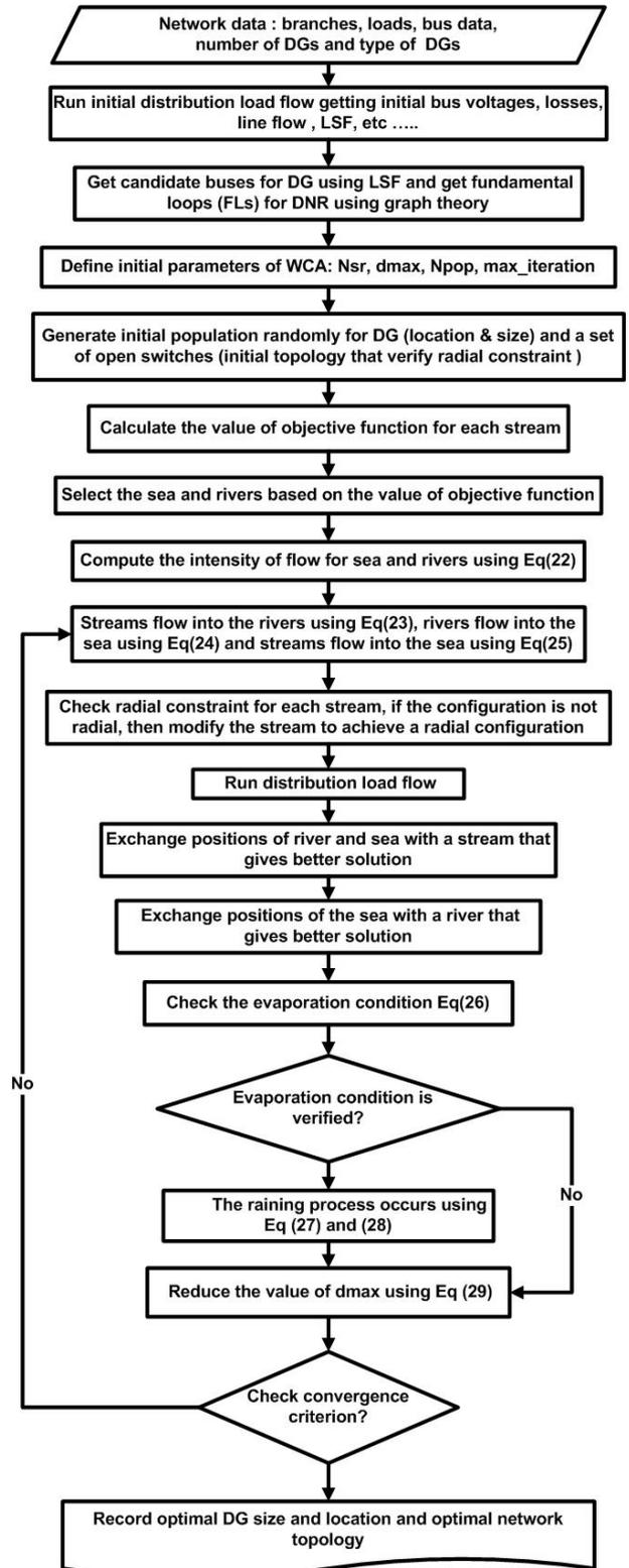
Fig. 3. Procedures for optimal DNR and DG allocation using the proposed WCA
