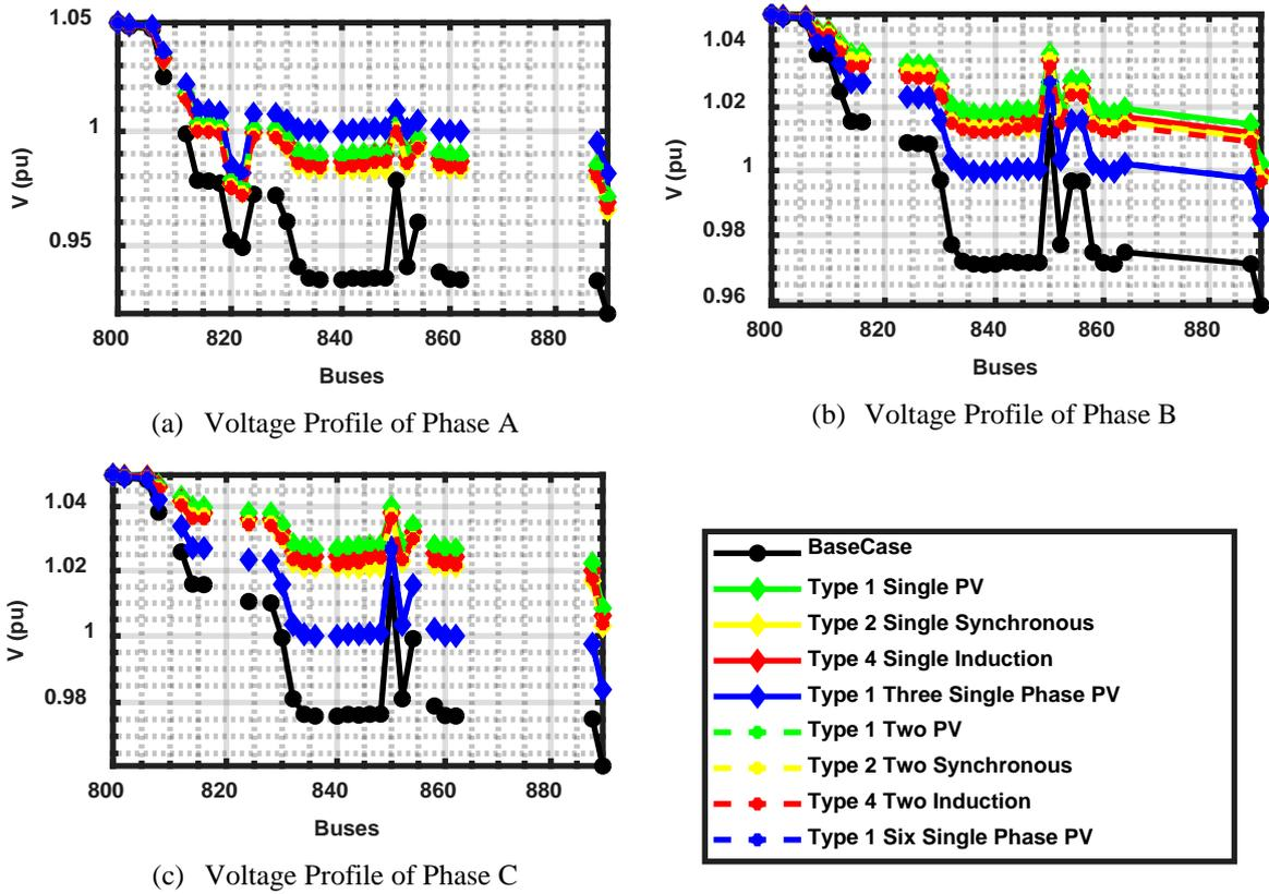
Fig. 6. Voltage Profile of Different DGs of the Three Phases for 34-Bus System by CSA
