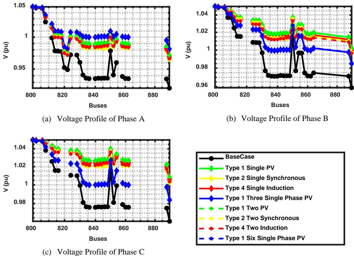
Fig. 7. Voltage Profile of Different DGs of the Three Phases for 34-Bus System by ABC
