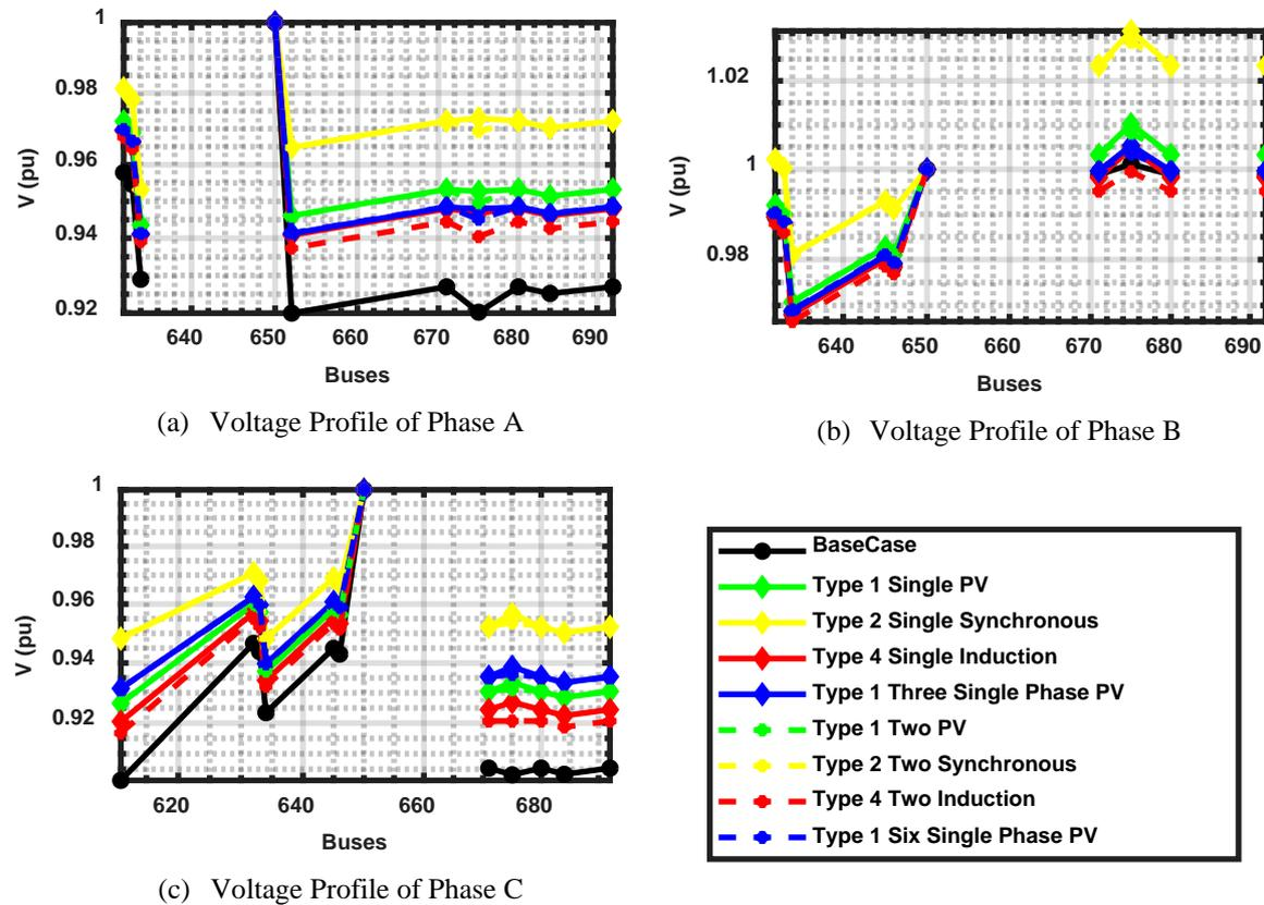
Fig. 5. Voltage Profile of Different DGs of the Three Phases for 13-Bus System by ABC
