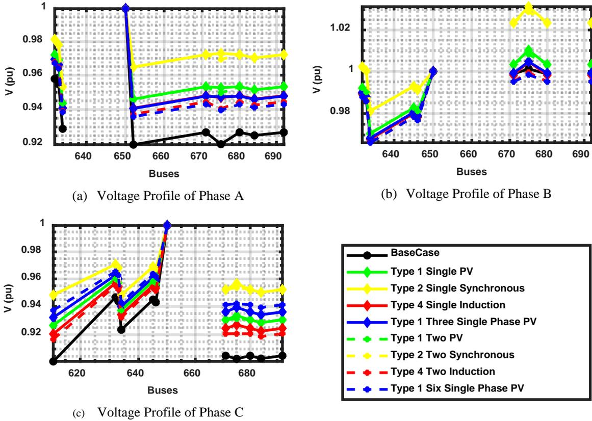
Fig. 4. Voltage Profile of Different DGs of the Three Phases for 13-Bus System by CSA
