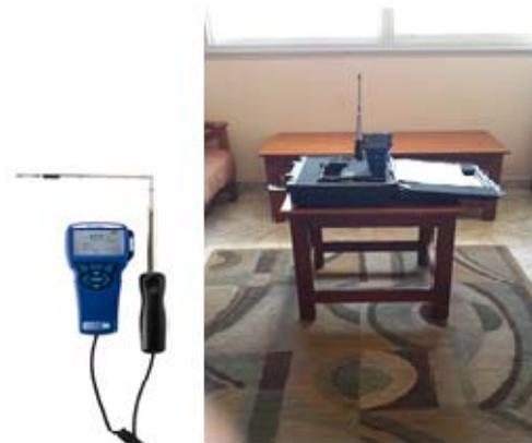
Fig. 6. Air velocity meter 9545-A and the field of study
