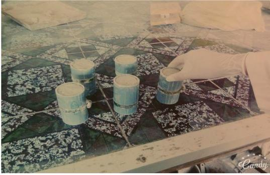
Photo (1): Soil samples during and after casting them in molds.
