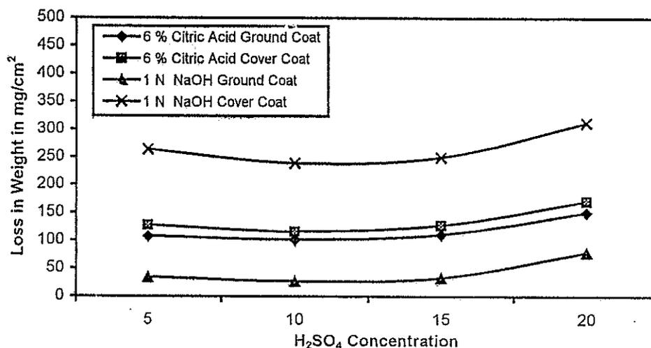
Figure 3: The Effect of Sulphuric Acid Concentration on both Base and Acid resistance of enamel
