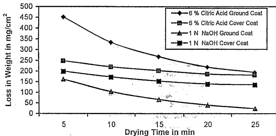
Figure1: The Effect of Drying Time on both Base and Acid resistance of enamel
