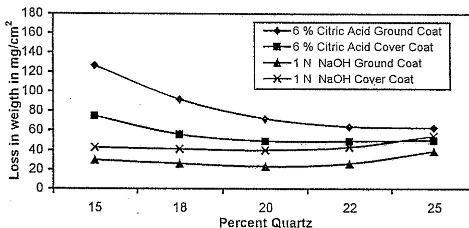
Figure 4: The effect of the Quartz Addition on both Base and Acid resistance of enamel
