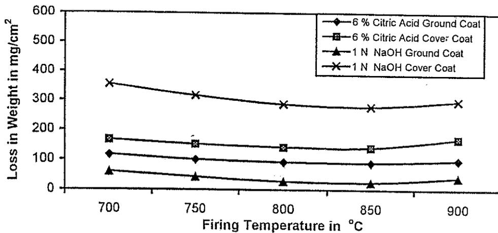
Figure 2: The Effect of Firing Temperature on both Base and Acid resistance of enamel
