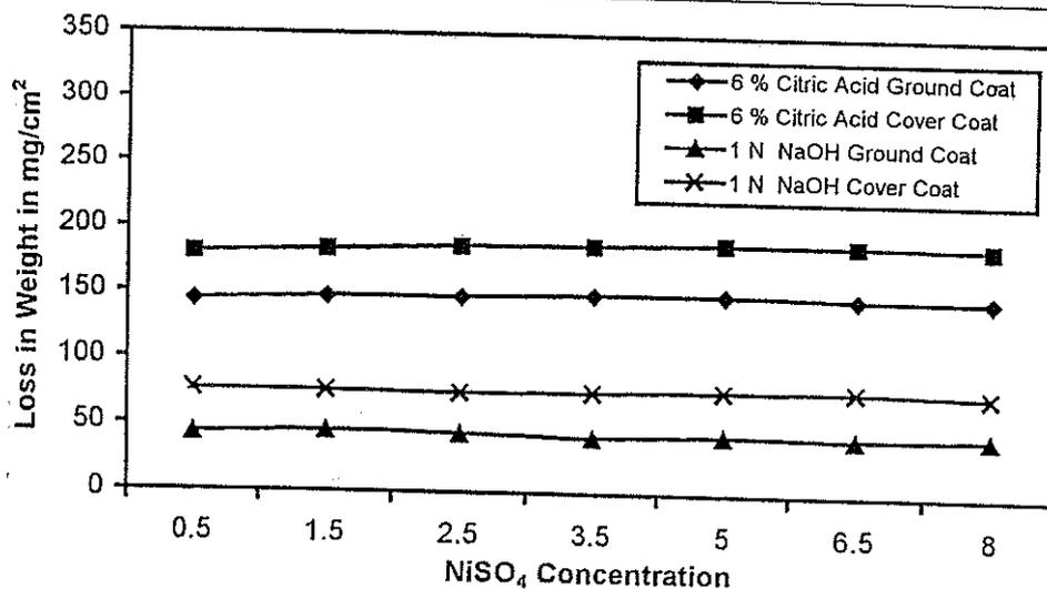
Figure 5: The Effect of the NiSO<sub>4</sub> Concentration on both Base and Acid resistance of enamel
