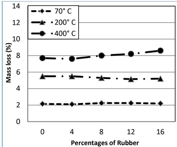
Fig. 18. Mass loss ratios of different concrete mixes after exposure to high temperatures
