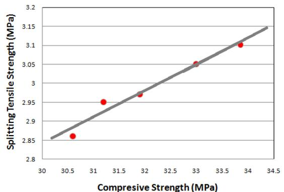
Fig. 7. Relation between compressive strength and tensile strength for crumb concrete.
