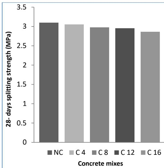
Fig. 5. Relation between percentages of crumb rubber aggregates and splitting tensile strength after 28 days.
