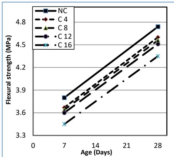
Fig. 8. Variation of flexural strength with different ages.
