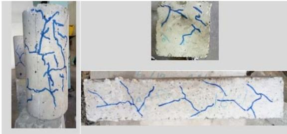
Fig. 10. Specimens after heating (400° C) in oven for two hours
