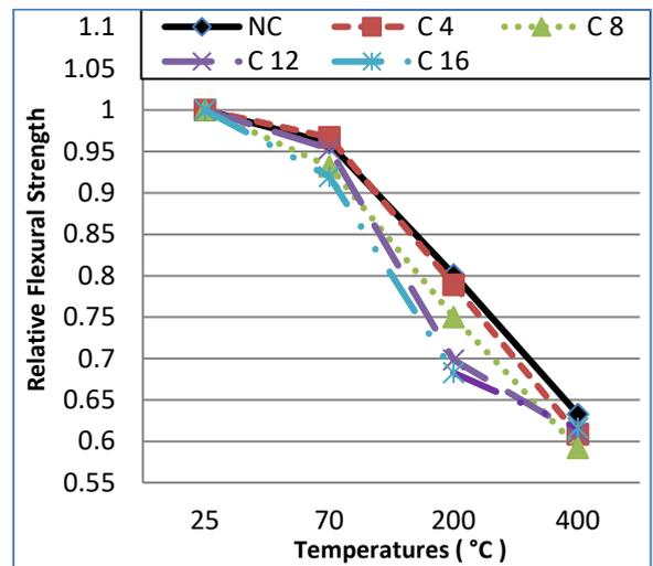
Fig. 17. Relative flexural strength versus temperature for concrete with different percentage of crumb rubber
