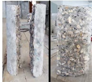
Fig. 6. Crumb concrete cylinder sample after splitting into two halves under splitting tensile test.
