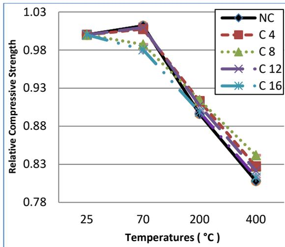
Fig. 13. Relative compressive strength versus temperature for concrete with different percentage of crumb rubber
