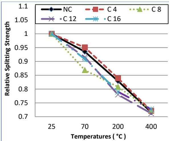
Fig. 15. Relative splitting tensile strength versus temperature for concrete with different percentage of crumb rubber
