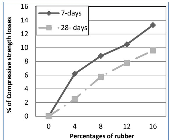
Fig. 4. The loss of compressive strength with different percentage of crumb rubber
