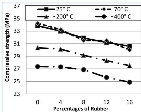
Fig. 11. Compressive strength versus rubber content at different temperature
