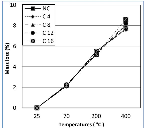
Fig. 19. Effect of high temperature on the mass loss of concrete containing different percentage of rubber
