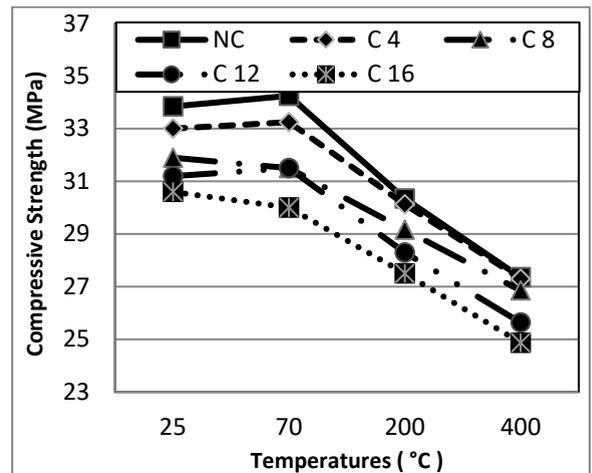
Fig. 12. Residual Compressive strength versus temperature for concrete with different rubber content
