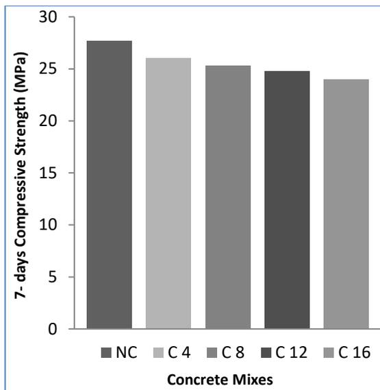
Fig. 2. Relation between percentages of crumb rubber aggregates and compressive strength after 7 days
