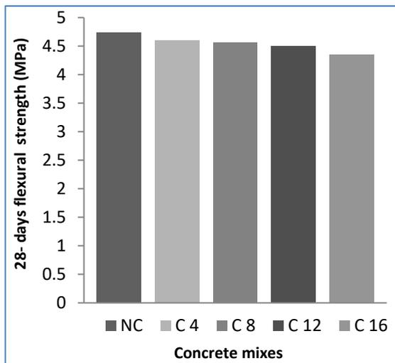
Fig. 9. Variation of flexural strength with different rubber content
