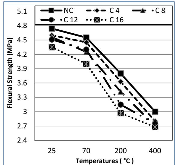
Fig. 16. Flexural strength versus rubber content at different temperature
