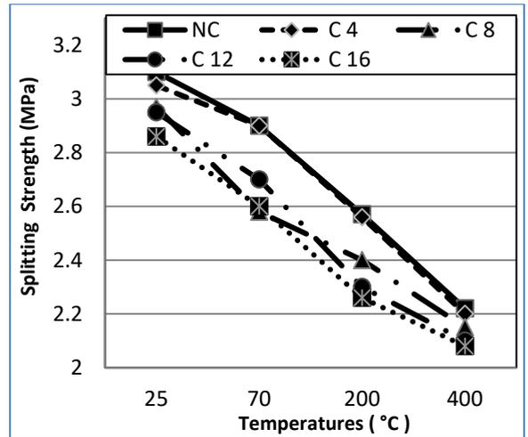
Fig. 14. Splitting Tensile strength versus rubber content at different temperature
