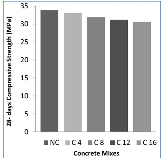
Fig. 3. Relation between percentages of crumb rubber aggregates and compressive strength after 28 days
