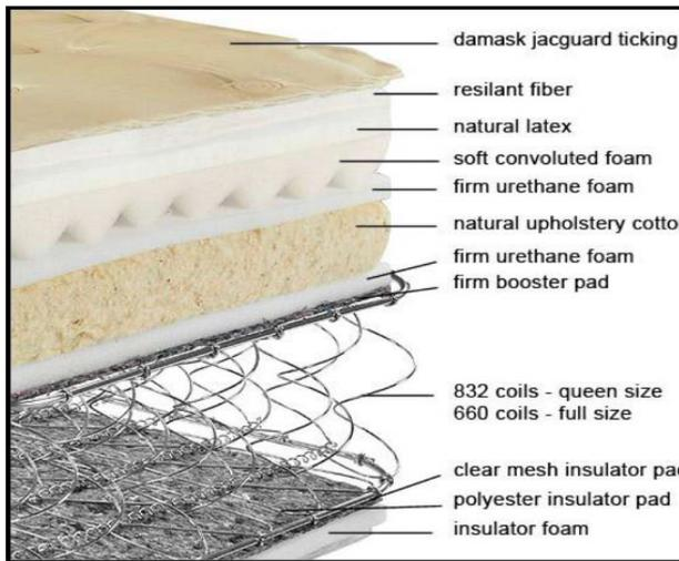
Fig (5): consists of innerspring mattress
