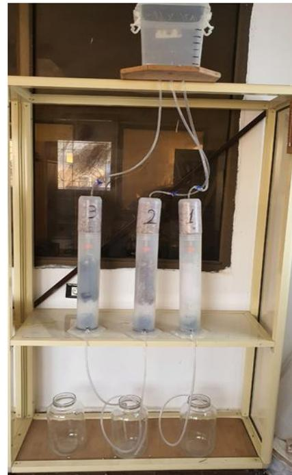
**Fig.(1). Schematic diagram of an elevation view of the wastewater treatment system.**
