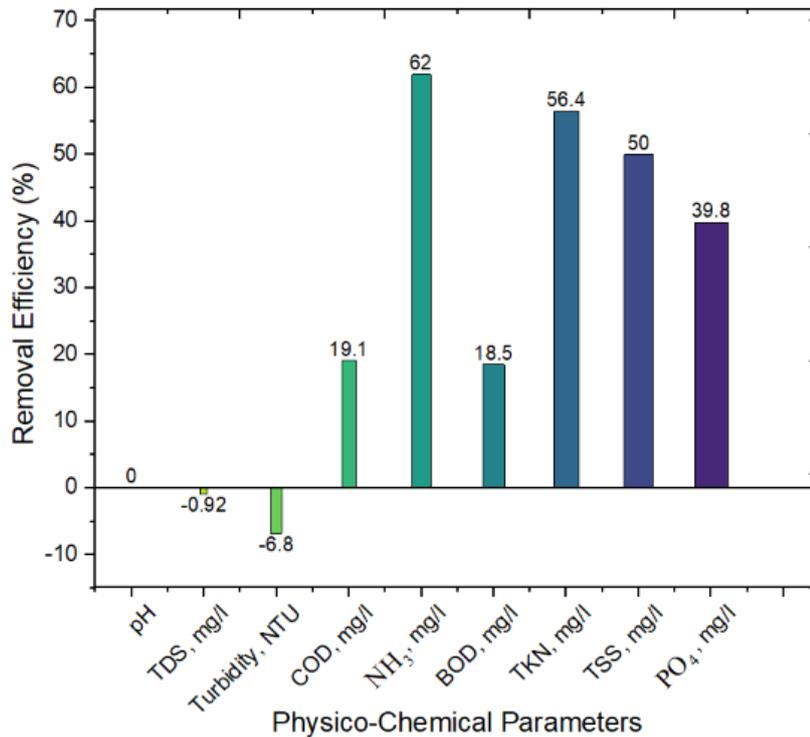
**Fig.(10). Parameters of water treated by activated carbon biofilter medium.**
