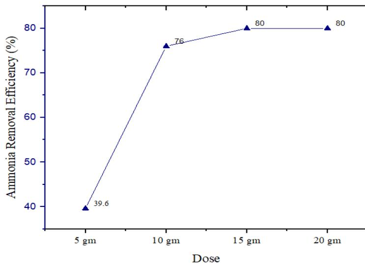
**Fig.(5). Medium doses of activated carbon biofilter medium.**
