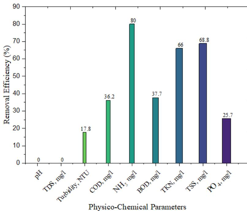
**Fig.(9). Parameters of water treated by activated carbon biofilter medium.**
