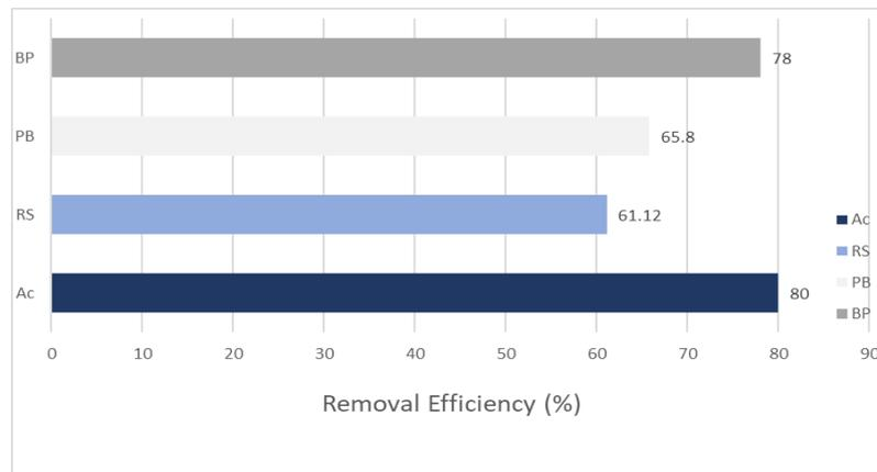
**Fig.(4). Removal efficiency (RE) of biofilter media while using G mechanical filter media.**
