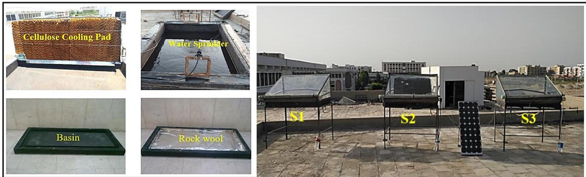
**Fig. (1): A photo of the three single slope solar stills and still components**
