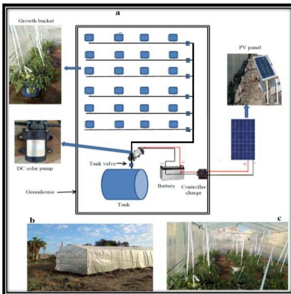
Fig. (1): Layout of pulsed deficit drip irrigation system in greenhouse powered by PV solar energy for cultivated tomato in bucket: a) Diagram of experiment components; b) Outside greenhouse; and c) Inside greenhouse.
