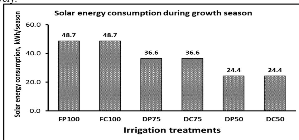
Fig. (10): Solar energy consumption for irrigating tomato crop in greenhouse.
