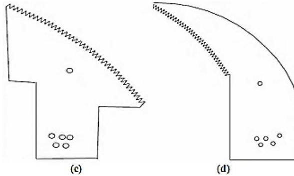
**Figure 3 (c) Backward curved serrated-edge blade, (d) forward-curved serrated-edge blade. (Mello and Harris, 2003)**
