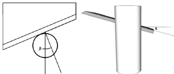
**Figure 4 Schematic diagram of a cutting blade design showing the blade oblique angle ( $\beta$ ) and tilt angles ( $\alpha$ ). (Quick, 1997)**
