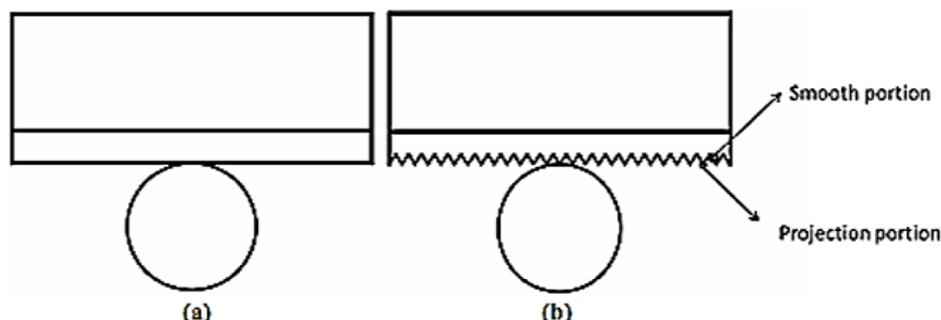
**Figure 2 (a) Cutting by the smooth-edged blade; (b) cutting by the serrated blade. (Frazzetta, 1988)**
