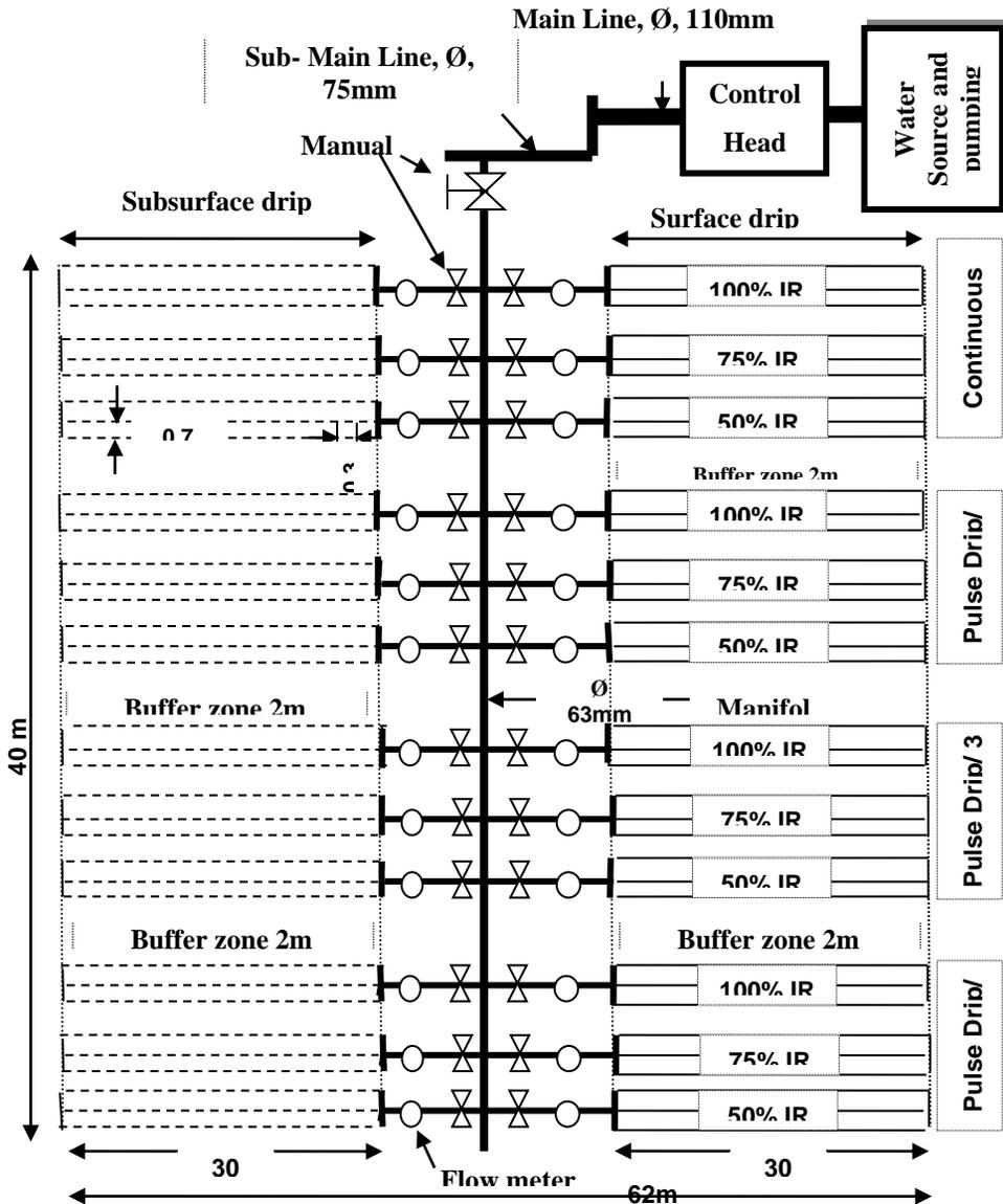
Fig. (2) Layout of irrigation systems with experimental design.
