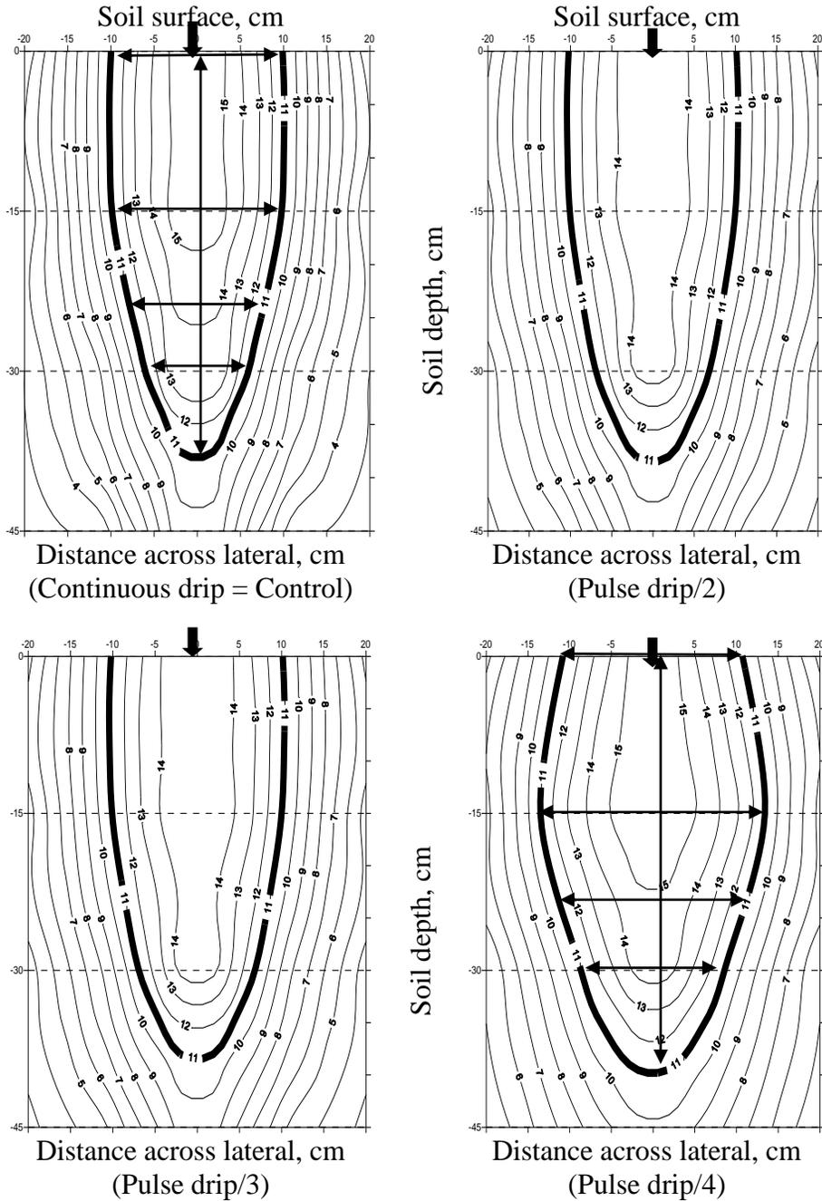
Fig.(6) Effect of pulse surface drip irrigation on wetted soil volume (more than or equal 100% of field capacity) at 75% from actual irrigation requirements
