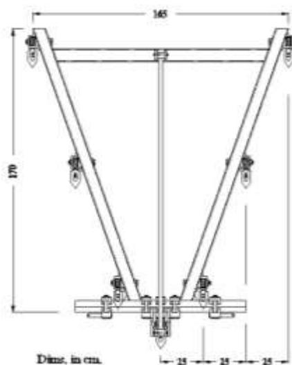
Fig. (2): Modified  $\Delta$ -shape chisel plow (4 rows).
