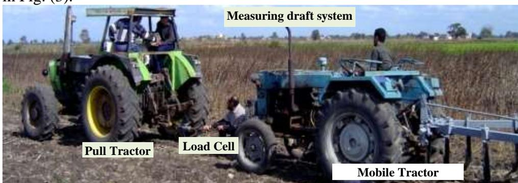
Fig. (3): Measuring draft force system during adjustment operation.
